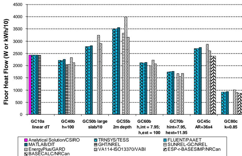
Figure 6. Selected BESTEST slab/ground heat transfer steady-state cases – after BESTESTing (Abbreviations along the x-axis are shorthand for the case descriptions; see Nomenclature section for label abbreviations; see Table 1 for legend description; see Neymark et al. [2008] full case descriptions.)
