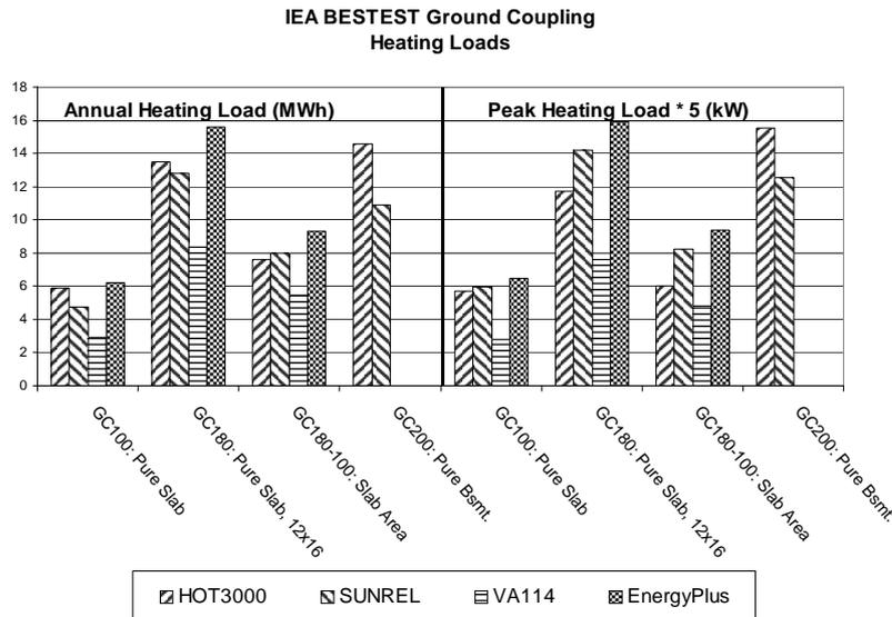
Figure 1. Results from IEA SHC Task 22 test cases isolating ground-coupled heat transfer effects (Deru et al. 2003)
