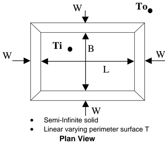
Figure 2. Schematic of CSIRO steady-state analytical solution case with rectangular geometry (Delsante et al. 1983; Spitler et al. 2001)
