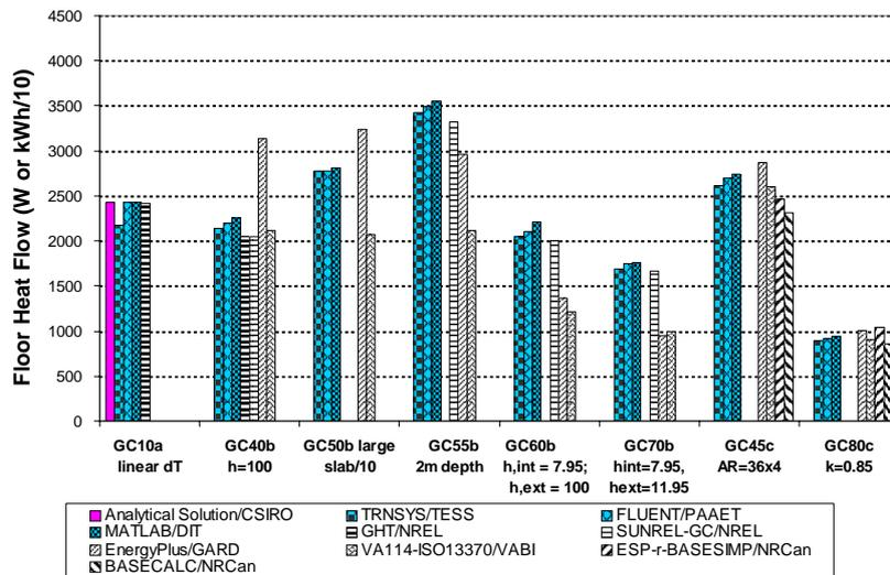
Figure 5. Selected BESTEST slab/ground heat transfer cases – floor conduction, before BESTESTing (Abbreviations along the x-axis are shorthand for the case descriptions; see Nomenclature section for label abbreviations; see Table 1 for legend description; see Neymark et al. [2008] full case descriptions.)
