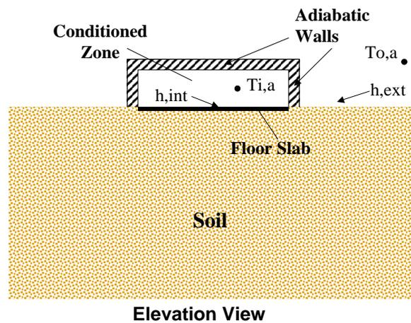
Figure 4. Comparative test base case schematic diagram – to isolate ground heat transfer
