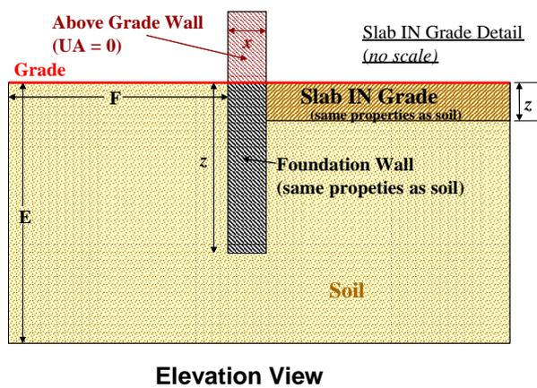
Figure 3. Slab-in-grade geometry idealization
