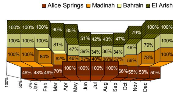
Figure 11 Monthly plant energy savings for system (B2) referred to a common active System (B). Note Alice Springs is in the Southern Hemisphere and cooler months are in the middle of the year.
