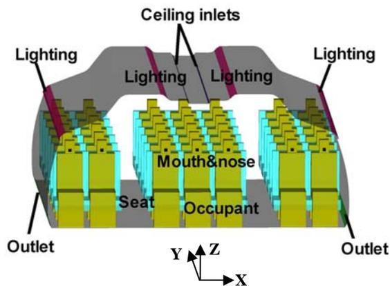
Figure 4 A current mixing air distribution system
