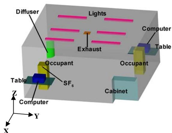
Figure 1 The office environment with displacement ventilation used for CFD validation
