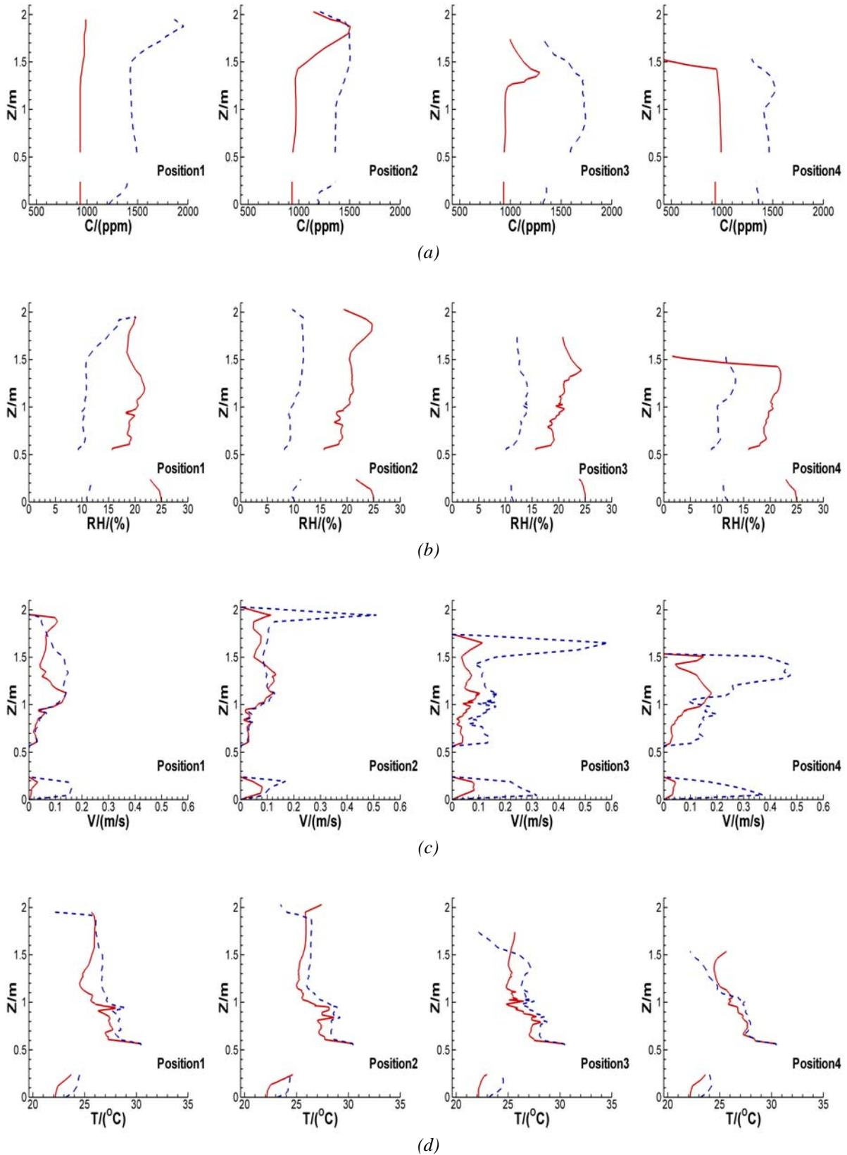
Figure 6 Comparison of CO<sub>2</sub> concentration (a), relative humidity (b), air velocity magnitude (c), and air temperature (d) in both cabin air systems at the four vertical positions: red solid lines for the new under-aisle displacement air distribution system, blue dashed lines for the mixing air system
