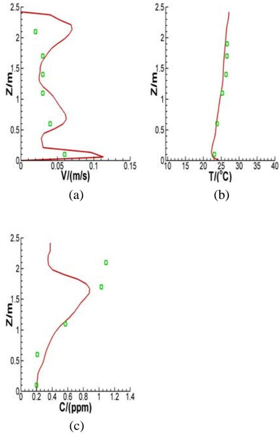
Figure 2 Comparison between the CFD results (lines) and experimental data (symbols) at the center of the office for air velocity, air temperature and SF<sub>6</sub> concentration along height
