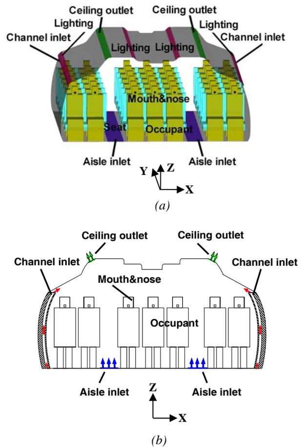
Figure 3 A section of a wide-body aircraft cabin model, (a) the new under-aisle air distribution system, (b) schematics of air supply scheme (sectional view)
