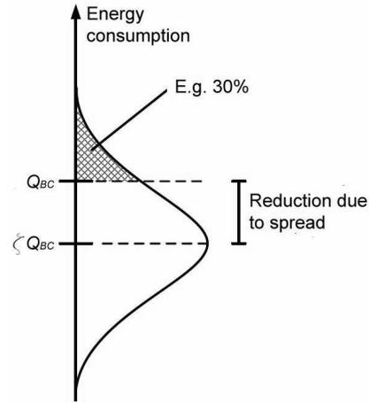
Figure 4 Building code's maximum energy consumption,  $Q_{BC}$ , reduced by factor  $\zeta$  to obtain a design energy consumption,  $\zeta \cdot Q_{BC}$ , to be applied for practical energy calculations.
