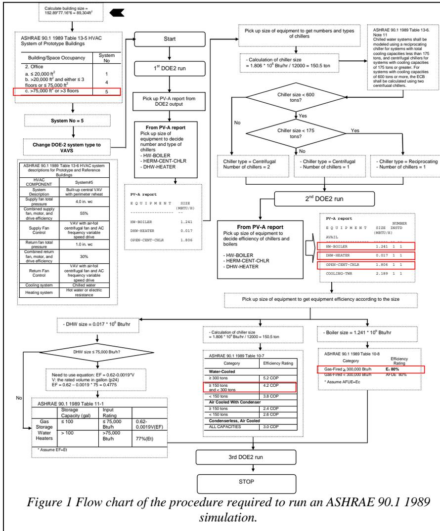
Figure 1 Flow chart of the procedure required to run an ASHRAE 90.1 1989 simulation.
