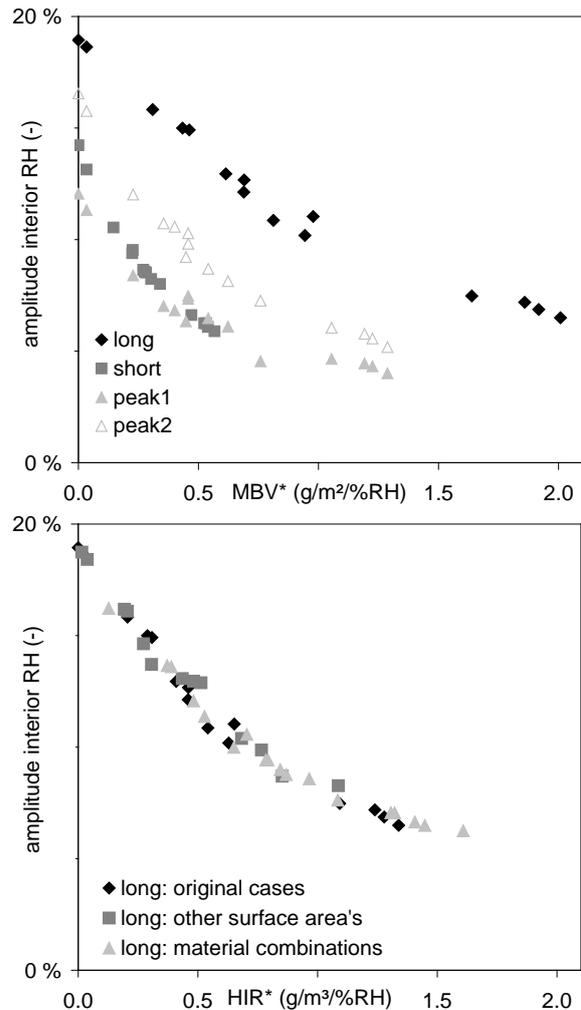
Figure 1 Relation between MBV\* and interior RH amplitude for the long, peak and short regimes (top) and relation between HIR\* and interior RH amplitude for the long regime (bottom).
