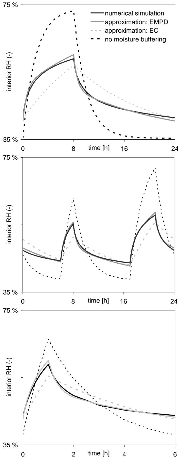
Figure 2 Comparison of interior RH variations simulated with the numerical model and with the EMPD and EC models, for the long (top), peak (middle) and short (bottom) moisture production regimes.
