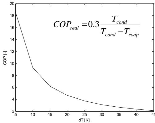
Figure 8 : Polynomial of the heat pump model
