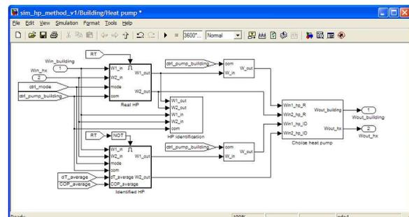
Figure 7 : Heat pump modelling (real and identified heat pump)
