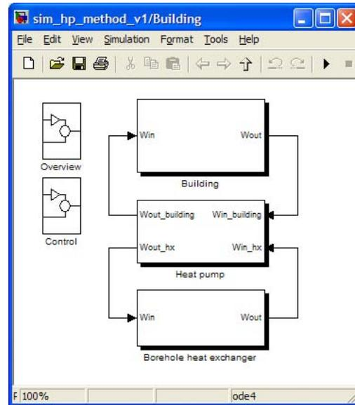
Figure 6 : First layer of the Simulink model of the complete GSHP system
