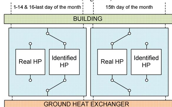
Figure 3 : Integration of real and simulated heat pump in the testing method
