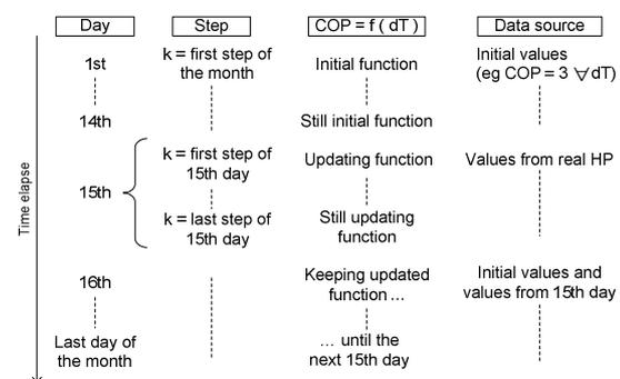
Figure 5 : Identification procedure for the heat pump
