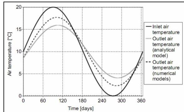
Figure 4: Response of the earth-to-air heat exchanger submitted to yearly sinusoidal solicitations
