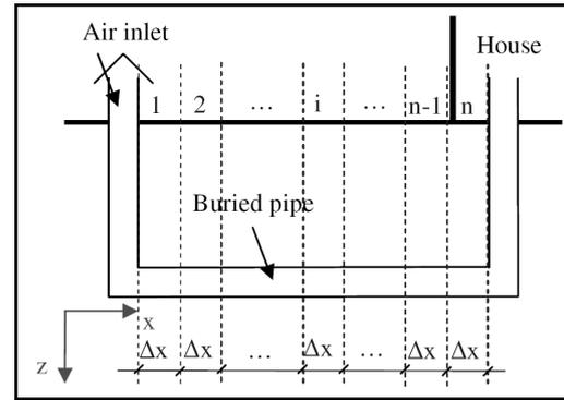
Figure 1: Discretization of the earth-to-air heat exchanger
