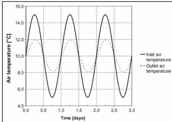
Figure 3: Response of the earth-to-air heat exchanger submitted to daily sinusoidal solicitations
