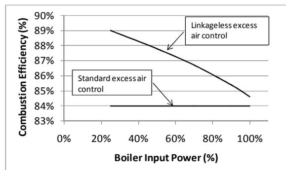
Figure 1. Typical combustion efficiency curves. The upper curve is taken from ASHRAE 2000.
