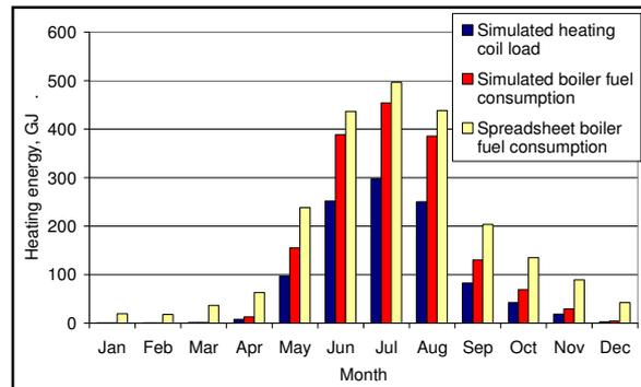
Figure 5: Comparison of simulation and spreadsheet fuel consumption.
