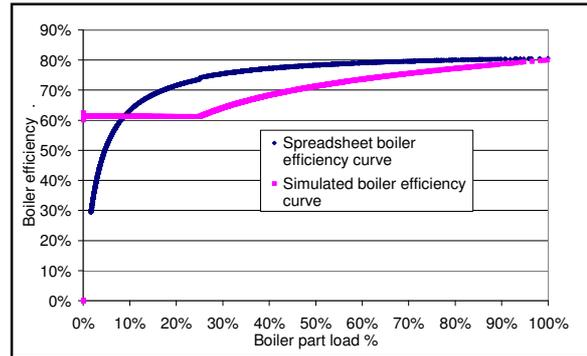
Figure 4: Boiler efficiency in the simulation and the spreadsheet
