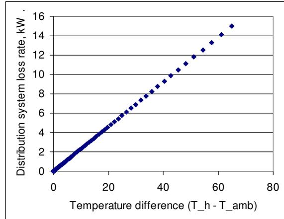
Figure 3: Distribution system heat loss rate as a function of the temperature difference between heating water and ambient.
