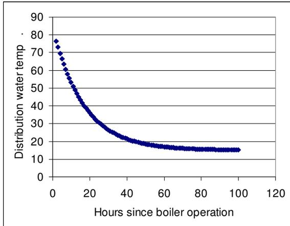
Figure 2: Temperature in the heating fluid distribution system.
