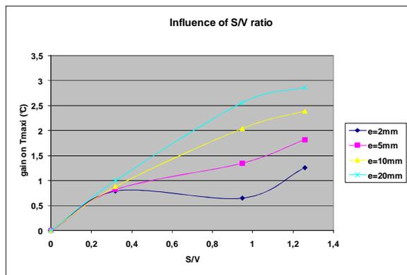
Figure 13: influence of the surface of PCM deployed, for different PCM thicknesses
