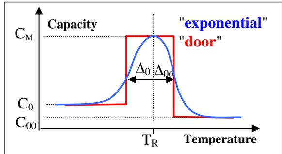
Figure 3 - Modelling of the heat capacity of a PCM in CoDyBa software
