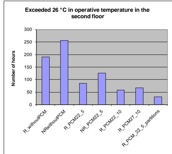
Figure 10 - Statistics on the number of hours for which 26°C are exceeded in the second floor during the whole summer
