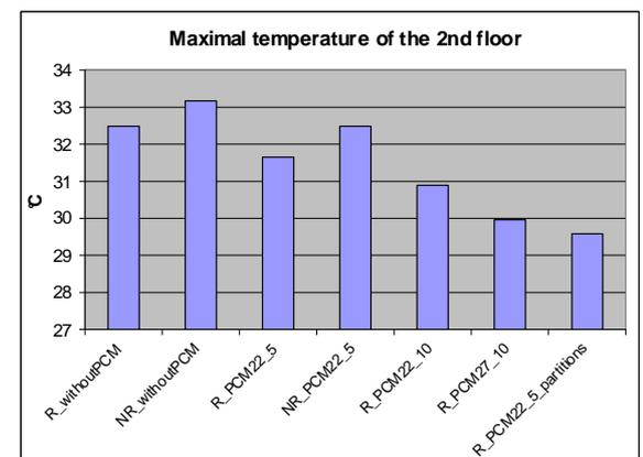
Figure 11 - Maximal temperature in the second floor during the whole summer
