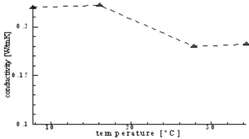
Figure 2 - Experimental PCM material thermal conductivity measured for several temperatures
