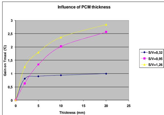
Figure 12: influence of the PCM thickness of PCM for 3 S/V ratios
