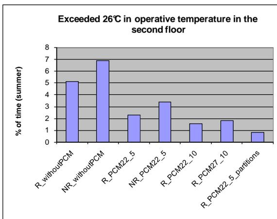
Figure 9 - Statistics on the percentage of time for which 26°C are exceeded in the second floor
