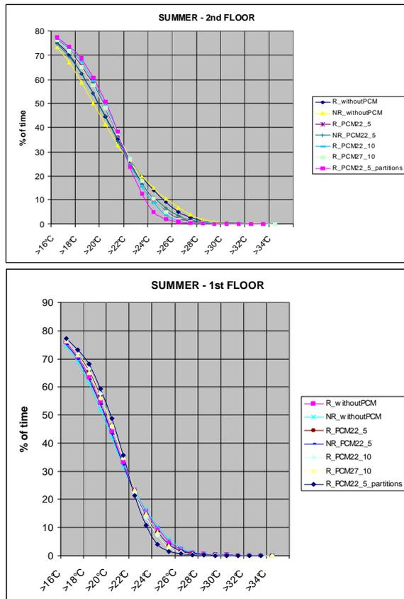
Figure 8 - Percentage of time for which a given temperature is exceeded on the full summer (1 May to 30 September)
