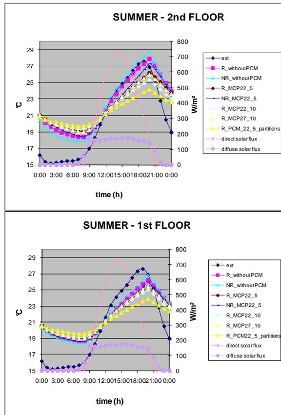
Figure 7 - Evolution of the temperature at ground floor (first floor) and the second floor one day in June in different conditions
