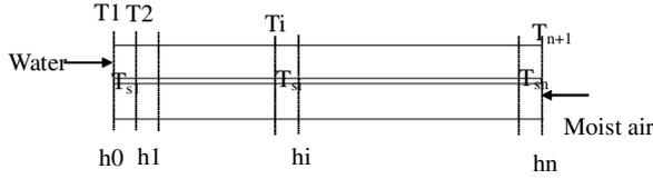
Figure 1 Calculation element of the heat exchanger surface
