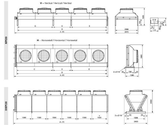
Figure 2 Front and side views of the dry cooler
