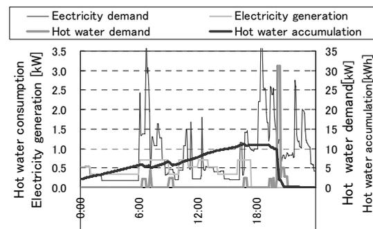
Figure 7 PEFC one day simulation result
