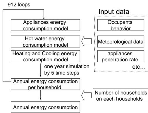
Figure 1 Simulation model flow chart
