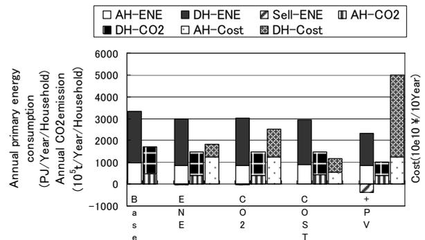
Figure 22 The effect of introducing the best systems (Left: Primary Energy Consumption, middle: CO<sub>2</sub> consumption, right: Cost)
