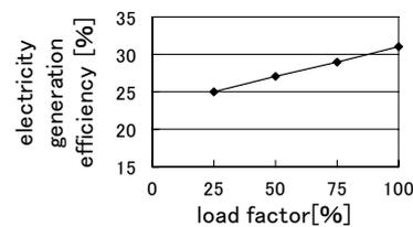
Figure 6 PEFC partial load characteristics
