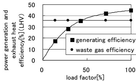
Figure 9 SOFC partial load characteristics
