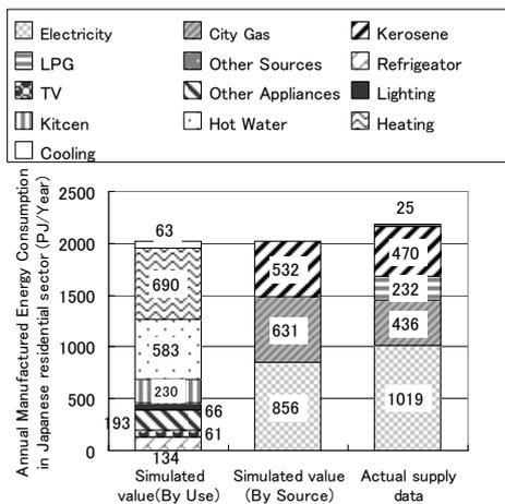
Figure 2 Simulated annual primary energy consumption and actual energy supply in Japan for 2005
