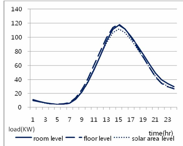
Figure 4: Cooling load comparison according to model resolution (kW)
