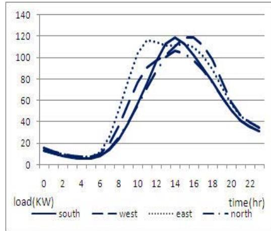
Figure 6: Cooling load comparison according to orientation (kW)
