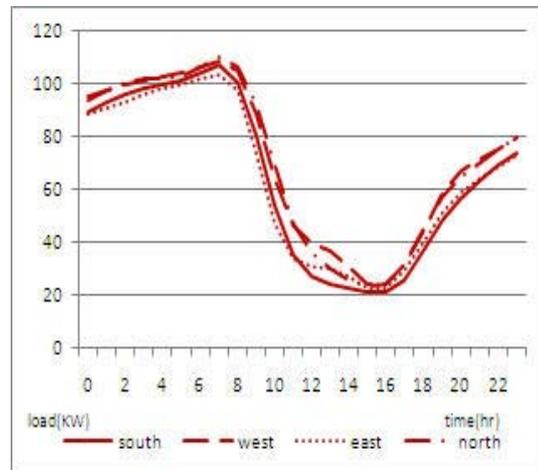
Figure 7: Heating load comparison according to orientation (kW)
