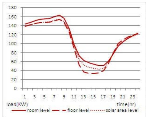
Figure 5: Heating load comparison according to model resolution (kW)
