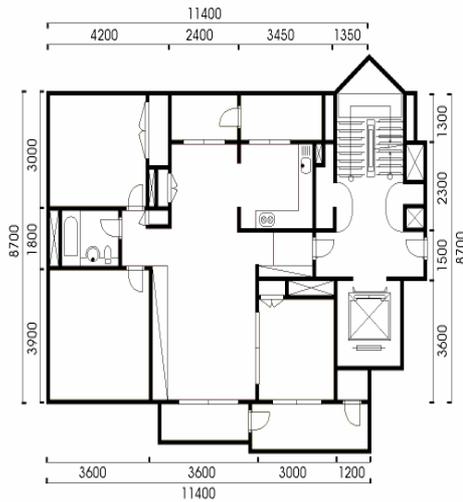
Figure 2: Floor plan of a single flat in a typical Korean apartment building
