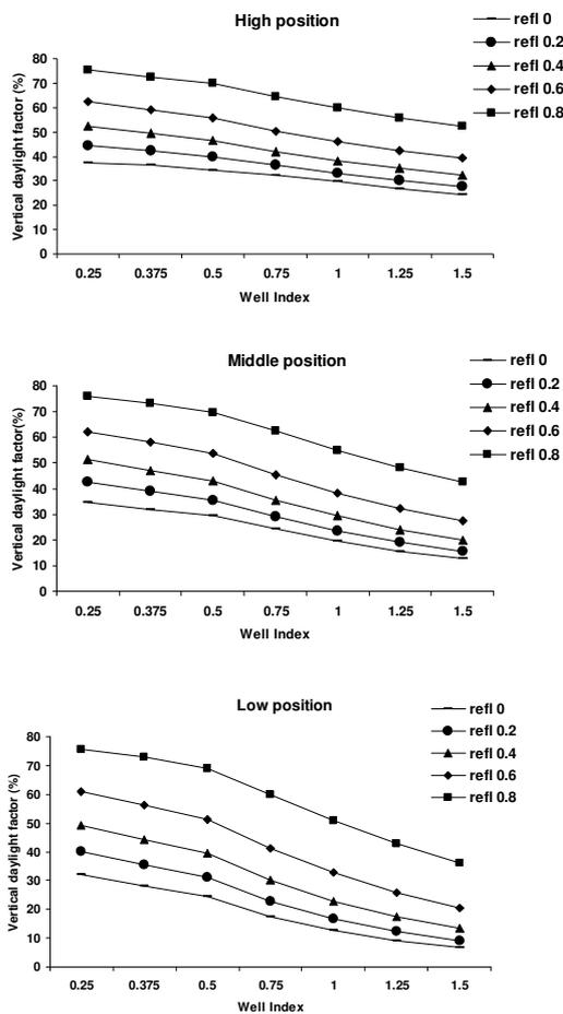
Figure 3: Simulated vertical daylight factor at the centre line of atrium wall.
