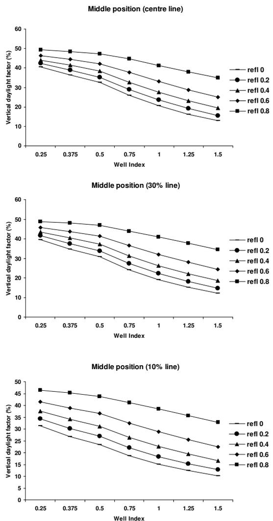
Figure 7: Simulated vertical daylight factor at the middle position of atrium wall.
