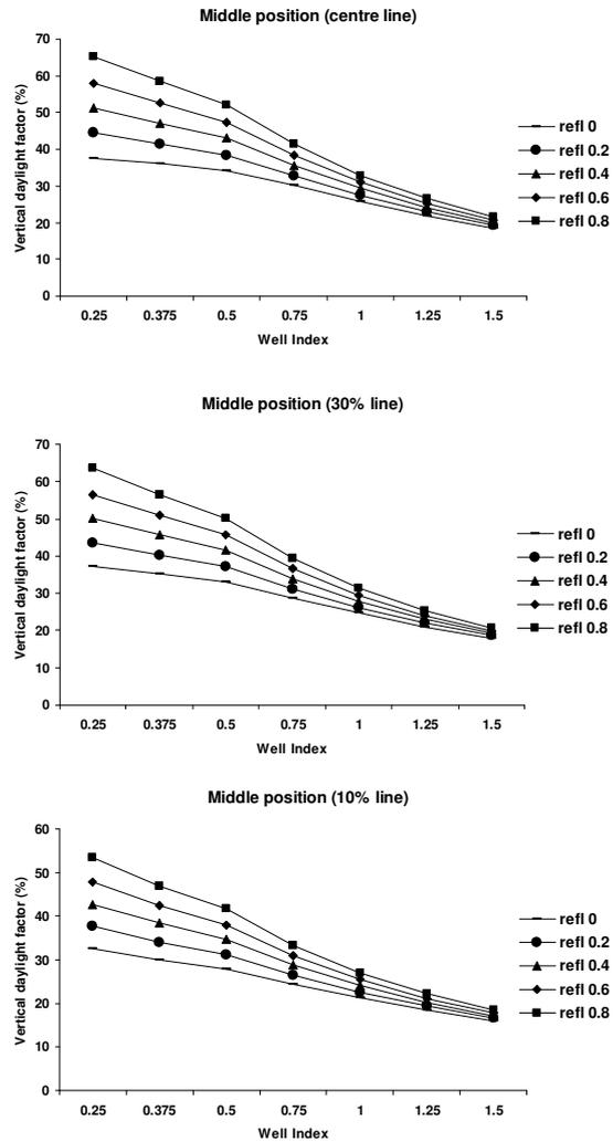
Figure 9: Simulated vertical daylight factor at the middle position of atrium wall.
