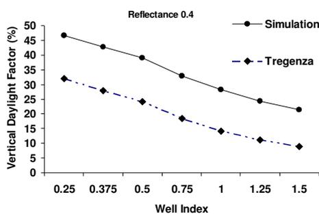
Figure 11: Comparison of average vertical daylight factor on the atrium wall.
