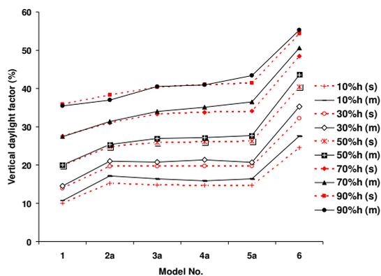
Figure 1: Comparison of vertical daylight factor between measurement (m) and simulation (s).
