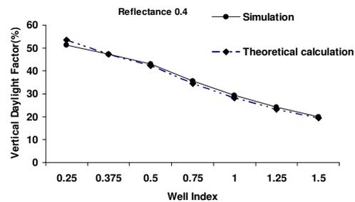
Figure 12: Comparison of vertical daylight factor at the centre line on the atrium wall.
