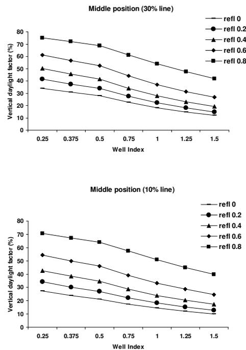
Figure 4: Simulated vertical daylight factor at the 30% and 10% line of atrium wall.
