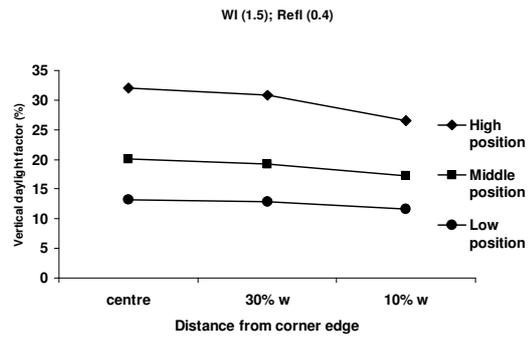
Figure 6: Vertical daylight factor distributions along the horizontal line (WI 1.5).
