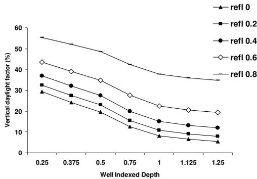
Figure 5: Vertical daylight factor at the centre line of atrium wall (WI 1.5).
