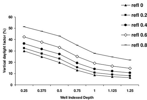
Figure 8: Vertical daylight factor at the centre line of atrium wall (WI 1.5).
