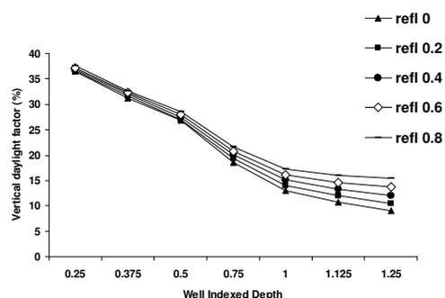
Figure 10: Vertical daylight factor at the centre line of atrium wall (WI 1.5).
