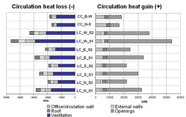
Figure 9 – Model 2: circulations heat gains and losses.
