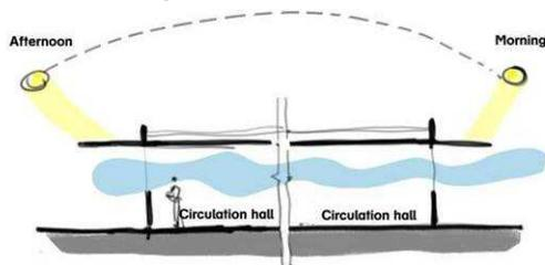
Figure 11 – Partial shading of both openings.
