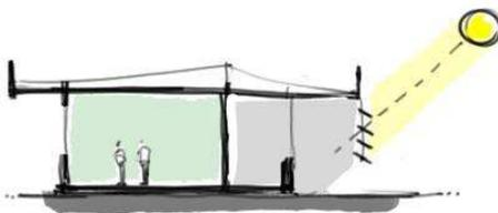
Figure 12 – Shading device for a West oriented circulation hall.
