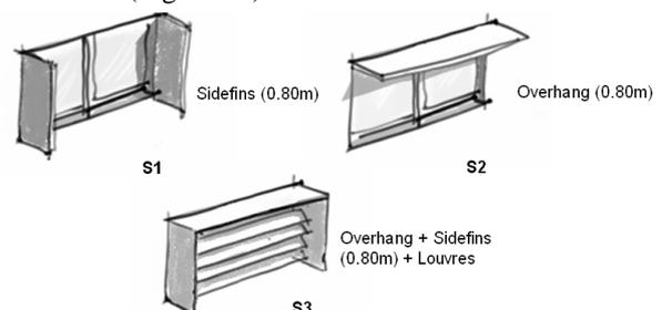
Figure 14 – Simulated shading devices.
