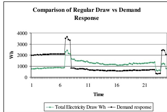
Figure 7 Comparison of regular electricity draw with the demand response to shift load to off-peak hours
