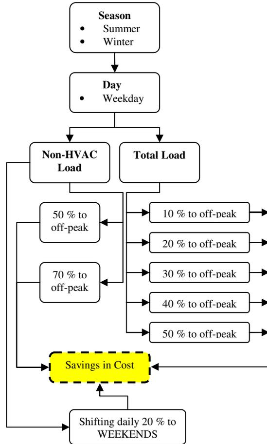
Figure 6 Flowchart showing different scenarios run with varying magnitude of demand response
