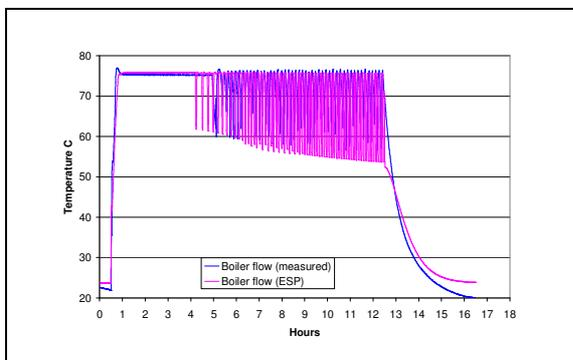
Figure 6 On/off thermostat boiler water temperature comparison.
