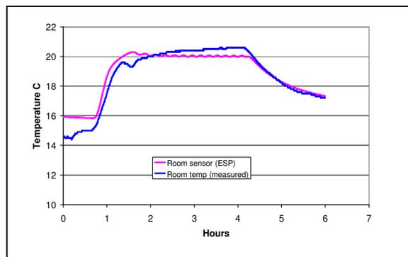
Figure 7 PI controller room temperature comparison
