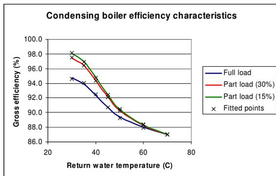
Figure 3 Efficiency characteristics for a condensing gas boiler.
