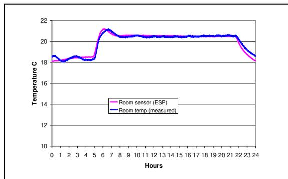
Figure 9 Time proportional PI controller room temperature comparison.
