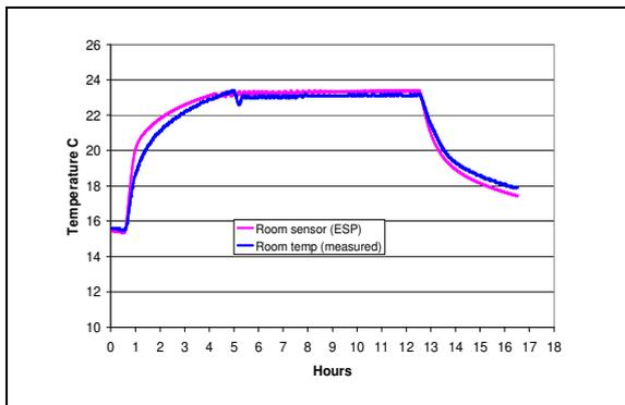
Figure 5 On/off Thermostat room temperature comparison (test room 1).
