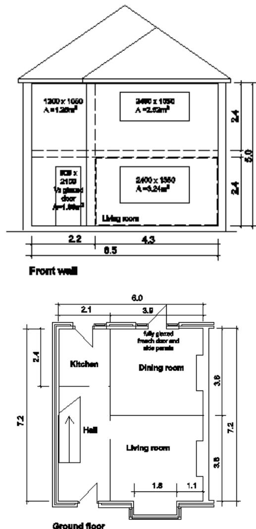
Figure 2 Elevation and ground floor plan for semi-detached house.
