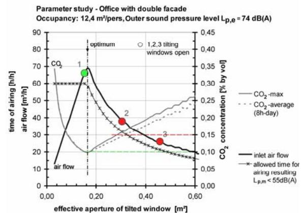
Fig. 8 – indoor air quality versus effective aperture in case of limited indoor sound pressure level
