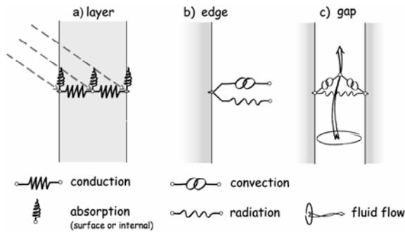
Fig. 2 - thermal and fluid flows
