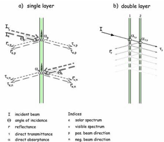
Fig. 3 - optical properties of single and double layer
