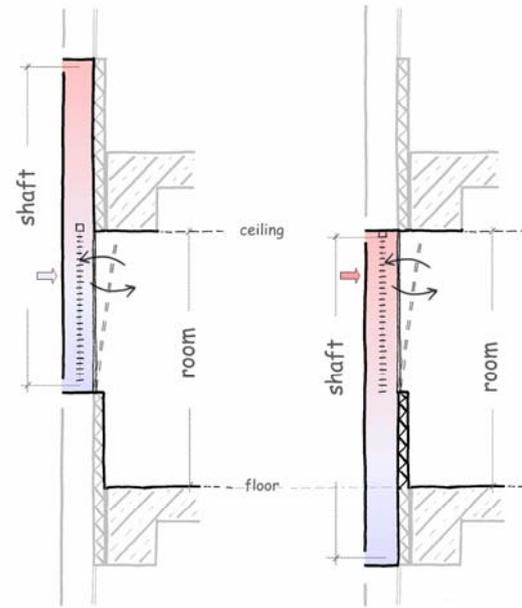
Fig. 9 - Room & shaft - staggered / matching levels
