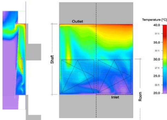
Fig. 15 3D-CFD of 'staggered shaft facade' at 500 W/m<sup>2</sup> insolation, shading closed
