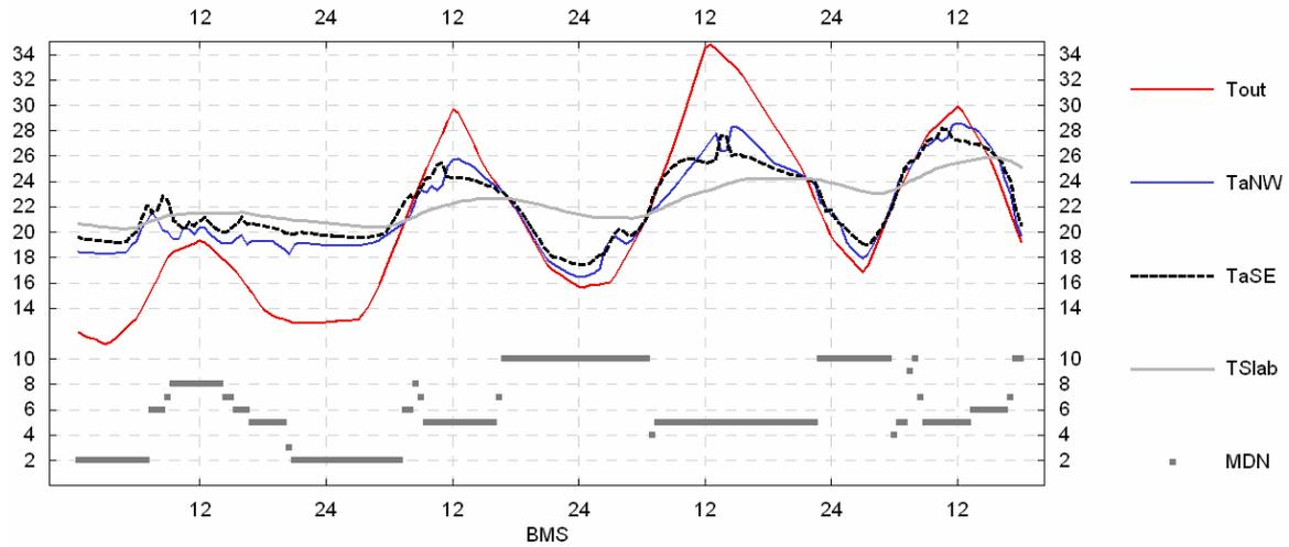
Figure 4. Performance of the natural ventilation system using the design sequence of operations embedded in EnergyPlus.  $T_{out}$  is the ambient temperature,  $T_{aNW}$  and  $T_{aSE}$  are the air temperatures in the perimeter zones on the north west and south east sides of the building and  $T_{slab}$  is the slab temperature at the position of the control sensor. MDN is the window opening mode number, as described in the text.
