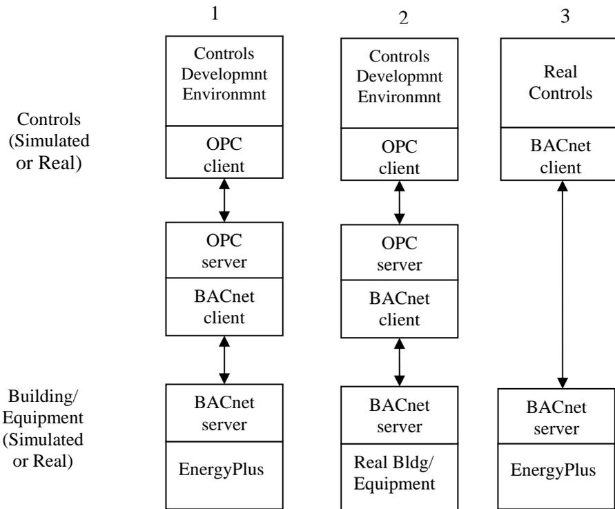
Figure 1. Configurations of the BCVTB for different development stages.
