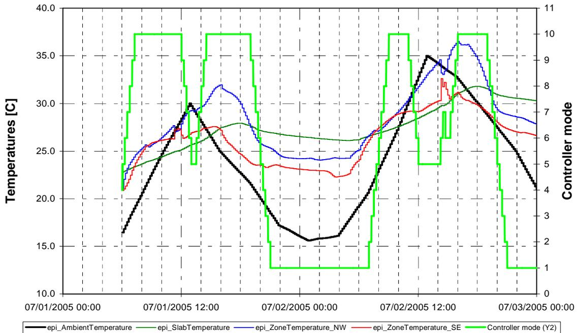
Figure 5. Performance of the natural ventilation system using an early version of the control program implemented in the hardware used in the building and connected to EnergyPlus. Controller mode is the window opening mode number, as described in the text.
