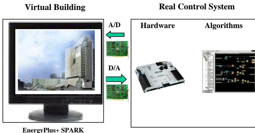
Figure 3. Configuration of used for hardware-in-the-loop testing of local loop controls.
