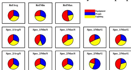
Figure 2 – Proportion of the total internal gain by component for each of the runs in the three approaches modelled.
