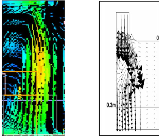
Figure 2 Airflow pattern from nozzle diffuser: simulation (left), literature (right)
