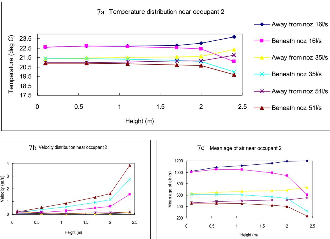
Figure 7 Temperature, velocity and mean age of air near occupant 2 (effects of diffuser location)
