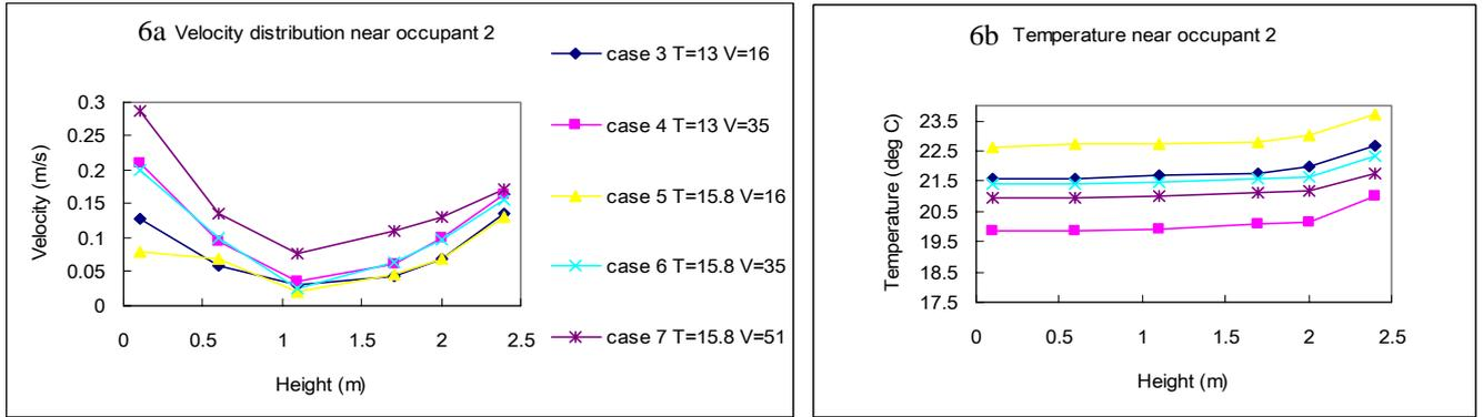
Figure 6 Velocity and Temperature near occupant 2 (effects of supply volume and temperature)
