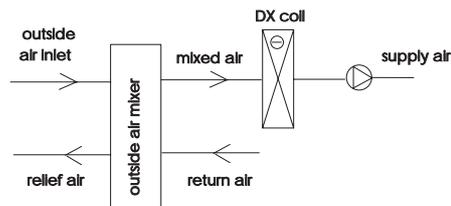
Figure 2 Air loop diagram of base configuration
