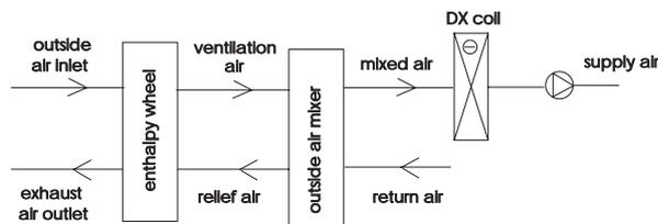
Figure 3 Air loop diagram of enthalpy wheel system
