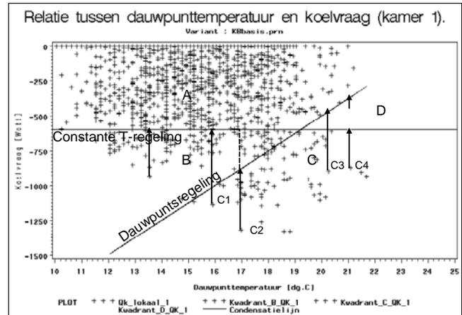
Figure 5 Cooling load versus dew point temperature
