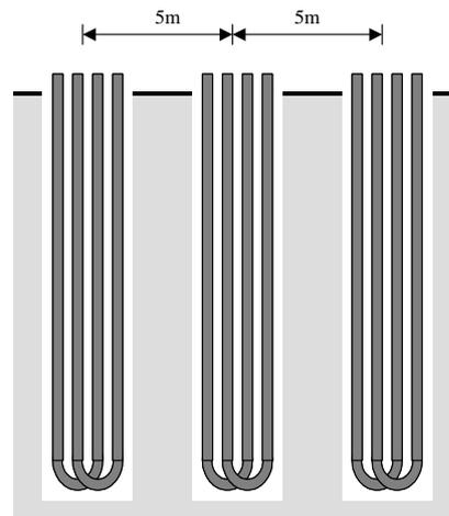
Figure 4 Bore hole and U-tube schematic
