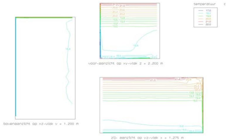
Figure 6 Temperature field in zone 1
