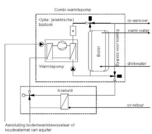
Figure 1 HVAC schematic layout
