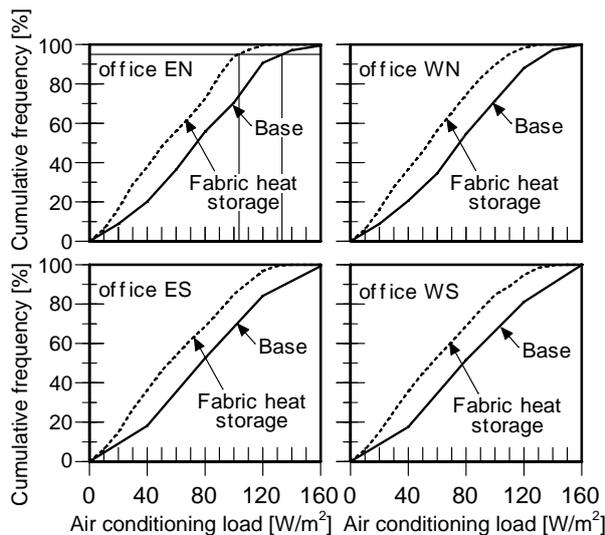
Figure 8 Comparison of cumulative frequency distribution of hourly air conditioner load in daytime
