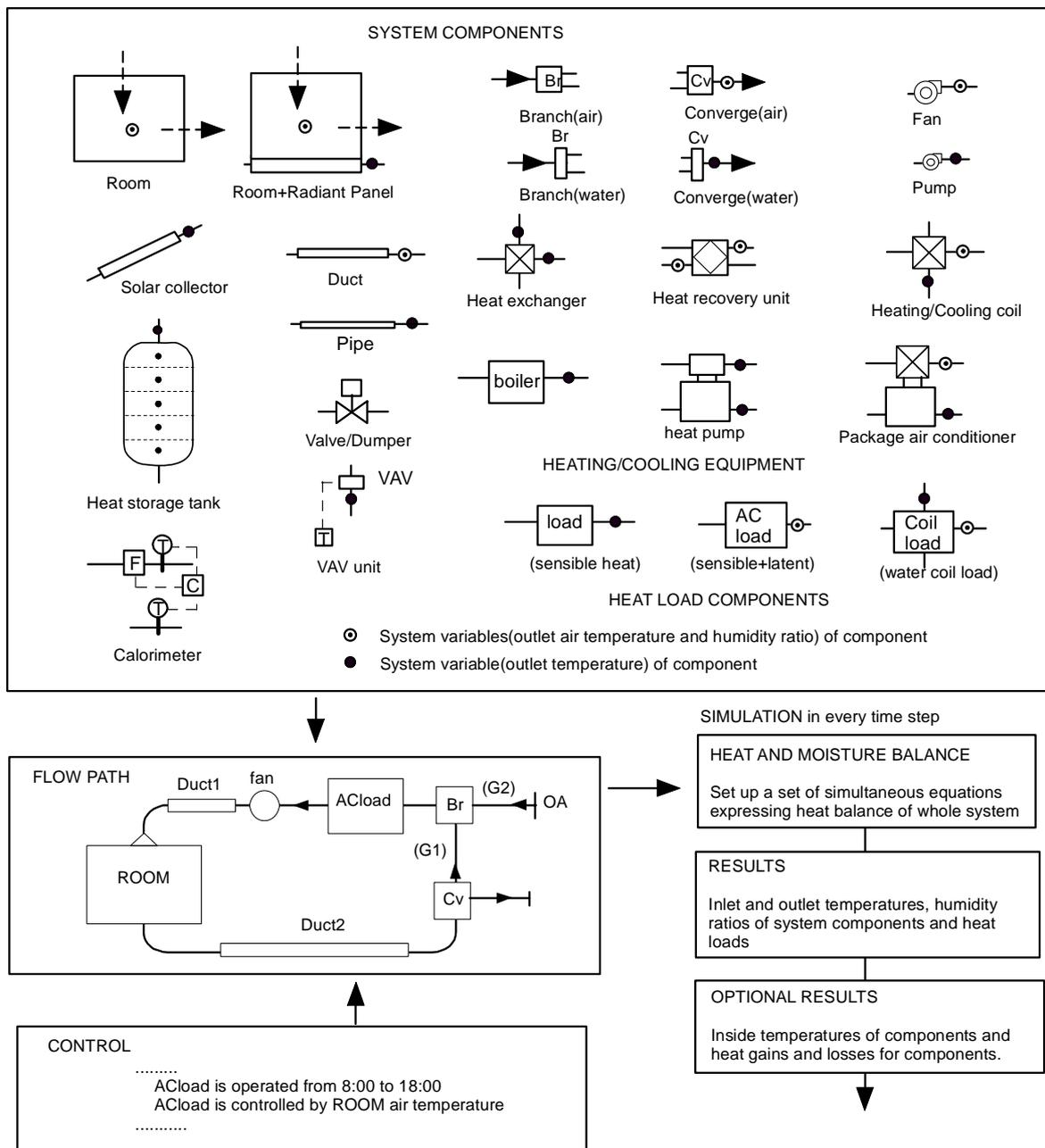
Figure 1 Simulation process in EESLISM
