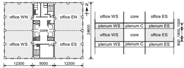
Figure 5 Floor plan and cross section of model building
