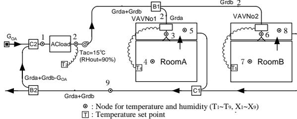
Figure 4 Simulation model for VAV system
