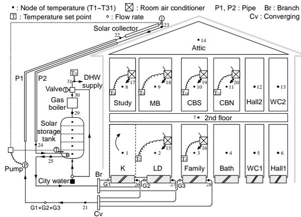
Figure 2 Simulation model for single solar family house
