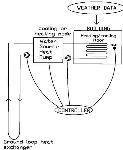
*Figure 3 Schematic diagram of the geothermal heat pump system components configuration*
