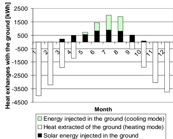
Figure 8 Heat exchanges with the ground during one year, the GHP works in heating or cooling mode and 12 m<sup>2</sup> of solar collectors are coupled with the boreholes
