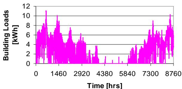
*Figure 2 Annual hourly building loads in heating mode for a 20°C indoor temperature considering typical climatic conditions for Chambéry (France)*
