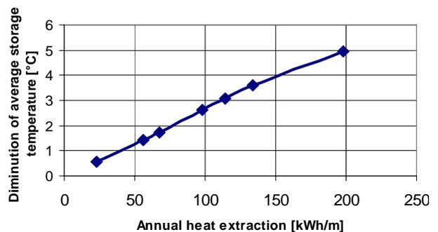
Figure 6 Diminution of the average storage temperature in function of annual heat extraction of the boreholes after 20 years of operation
