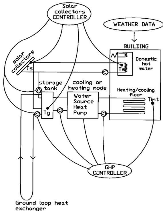
Figure 7 Schematic diagram of the coupling of solar collectors with geothermal heat pump system
