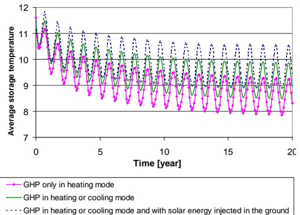
Figure 4 Evolution of the ground storage temperature
