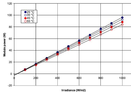
Figure 2 - Power as a function of irradiance. Data from Kenny *et al.*, 2003.
