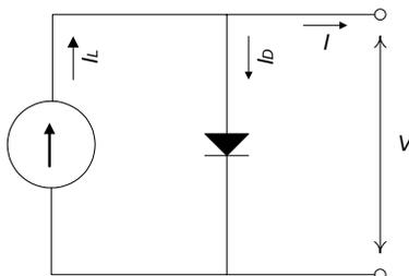
Figure 4 – Equivalent one-diode circuit in ESP-r.
