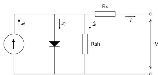
Figure 6 – Proposed equivalent one-diode circuit.
