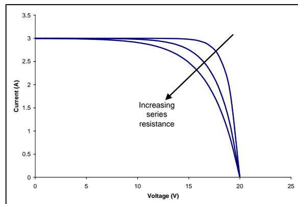
Figure 5 – Effect of series resistance on the I-V characteristics of a solar cell.
