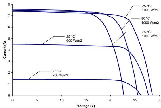
Figure 1 – PV module I-V curves.
