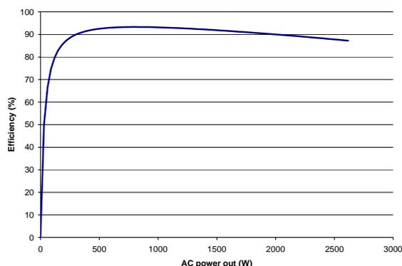
Figure 7 – Typical inverter efficiency curve.
