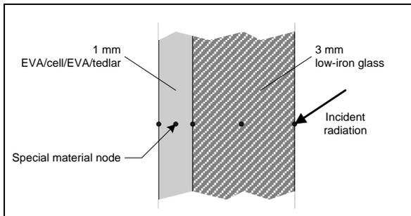
Figure 3 – ESP-r model of a PV module.
