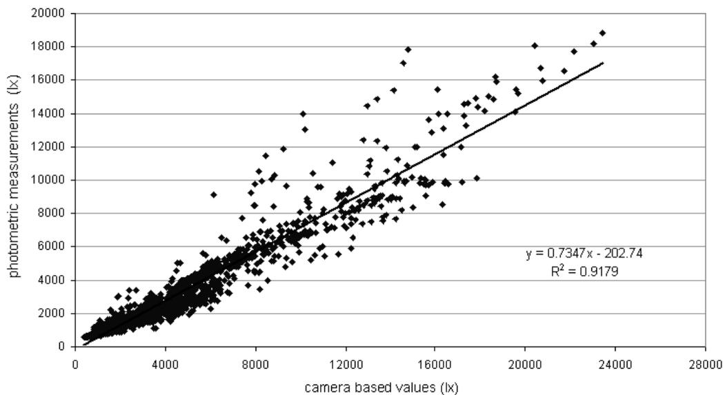
Figure 7 Photometrically measured versus camera-based illuminance values
