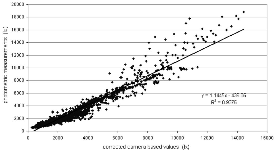
Figure 8 Photometrically measured versus corrected camera-based illuminance values
