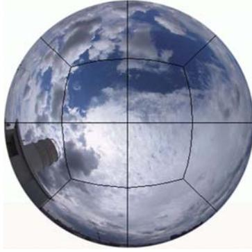
Figure 4 Projection of 12 sectors on a fisheye image
