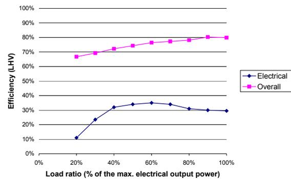
Fig. 1: electrical and overall efficiency characteristic curve of a 1 kW<sub>el</sub> natural gas fired SOFC system (according to (Erdmann, 2002) and adapted according guidelines of (Krewitt et al., 2004))
