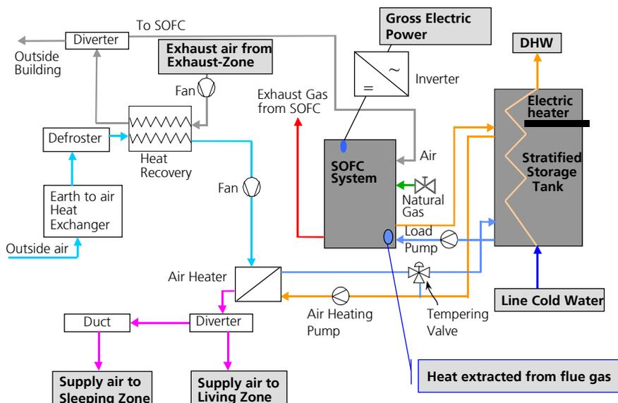
Fig. 5: Ventilation system with integrated SOFC for supplying heat and electricity to HPB.
