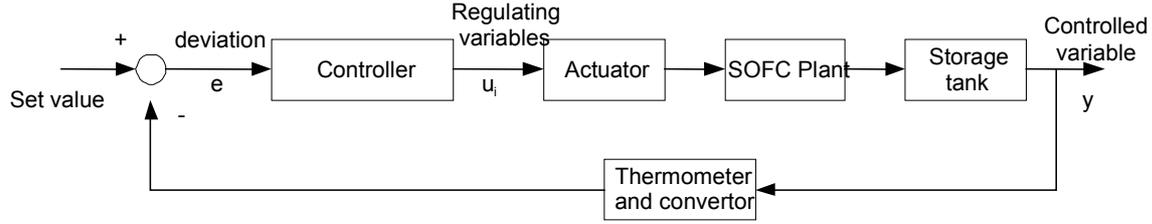
Fig. 2: Flowchart of control loop
