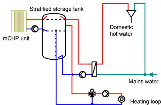
Fig. 4: Schematic diagram of the HVAC system
