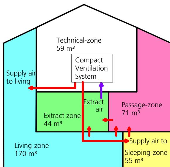
Fig. 3: Building with five zones and air flow paths of ventilation system (Ullah, 2004)
