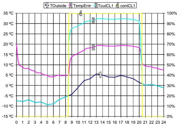
Figure 20 Behaviour of the same AHU in a “very cold” day and double boilers heating power
