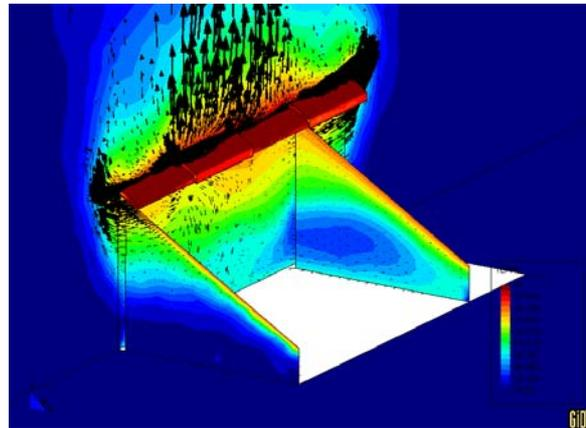
Figure15. CFD simulations, series 3. Temperature contours and velocity vectors in absence of wind.
