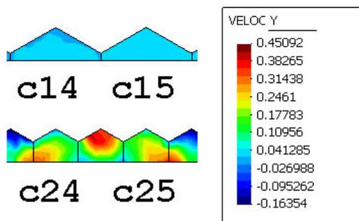
Figure13. Wind velocity module (m/s) in Haima's section with curtains at the entrance.
