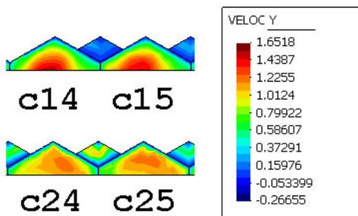
Figure14. Wind velocity module (m/s) in Haima's section with absence of curtains at the entrance.
