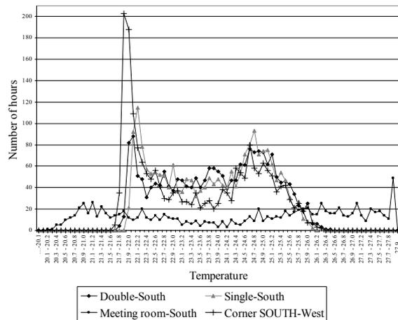
Figure 6. Directed operative temperatures for the 30% glazed building (south orientation).
