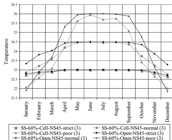
Figure 3. Weighted air temperatures for the 60% glazed building (third alternative).
