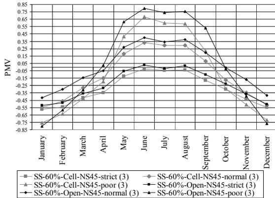
Figure 4. Weighted average PMV for the 60% glazed building (third alternative).
