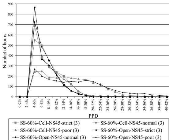
Figure 5. Number of working hours for certain average PPD for the 60% glazed building (third alternative). PPD can not be below 5 %, although the results from IDA says so.
