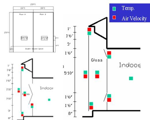
Figure 6 Plan and Section of the Full scale mock up
