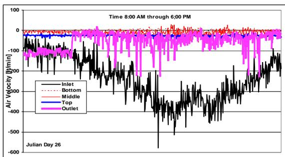
Figure 17 Airflow through the FSM of the DSF
