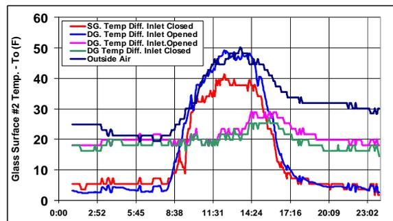
Figure 15 Glass surface temperature difference with respect to outside air in December
