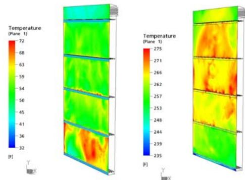
Figure 20 CFD model of DSF using measured boundary conditions for open inlets winter (left) and closed inlets summer (right) seasons.
