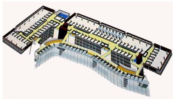
Figure 4 Atrium and Laboratory thermal zones
