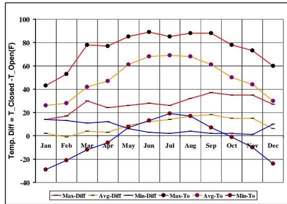
Figure 9 Outdoors temperature and difference in T within the DSF as a function of inlets' position.
