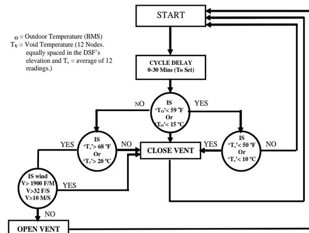
Figure 8 Airflow logic control for inlets operation
