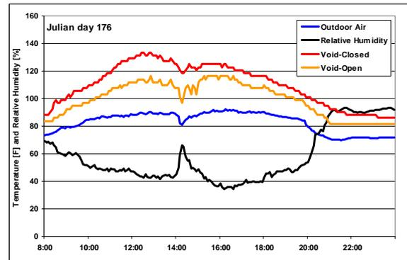
Figure 10 Temperature and humidity outside and within DSF void as a function of time (J- day 176)
