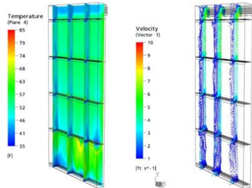
Figure 19 CFD model of DSF wall using measured winter boundary conditions for Temp and Wind.
