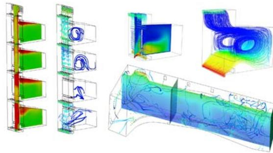
Figure 3 CFD models of DSF, Atrium and Offices
