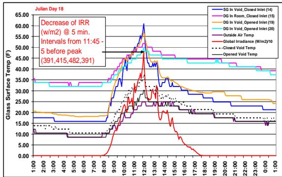
Figure 16 Glass surface temperatures at the time of its breakage due to sudden drop of  $\sim 100$  W/m<sup>2</sup>
