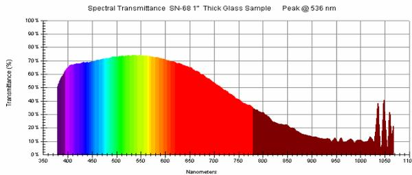
Figure 11 Spectral transmittance of the glass
