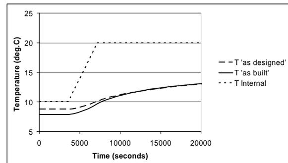
Figure 7. Comparison of internal surface temperature
