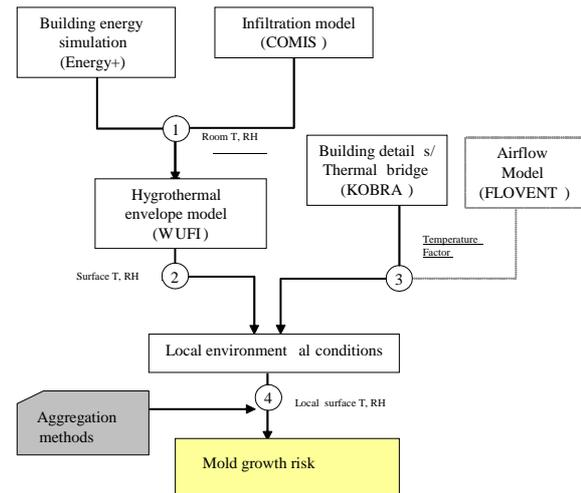
Figure 1 Flowchart of mixed simulation approach
