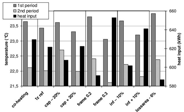
Figure 6 Sensitivity analysis: average temperature during first and second period, calculated heat input
