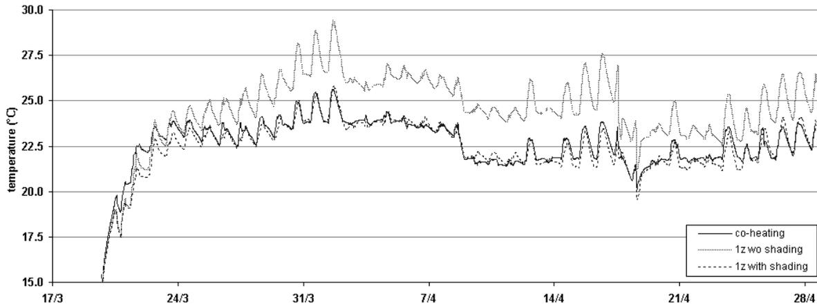
Figure 3 Temperature profile in the building: simulations with a single zone model
