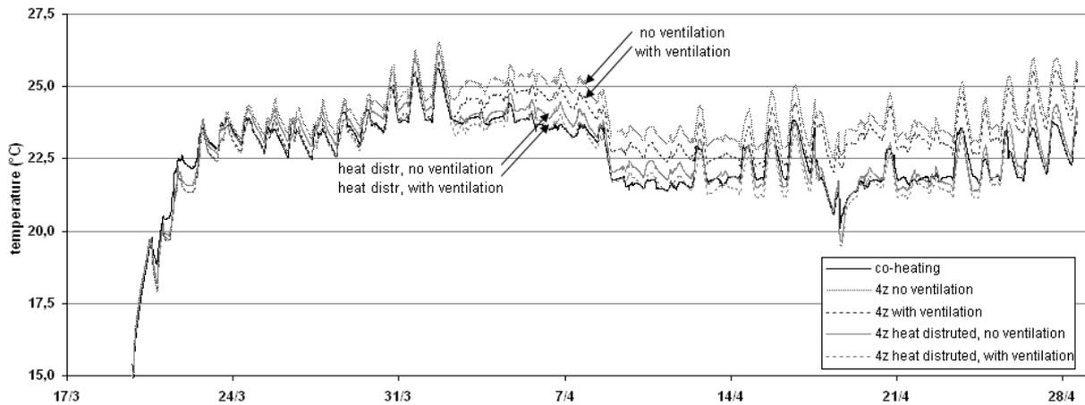
Figure 4 Temperature profile in the building: simulations with a multi zone model
