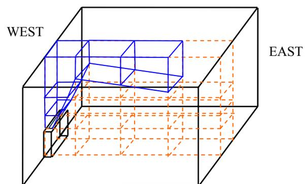
Figure 1 Zonal partitioning of a room containing a vertical jet
