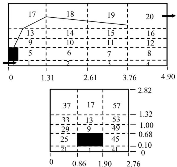
Figure 3 Zonal partitioning for the plan containing the jet
