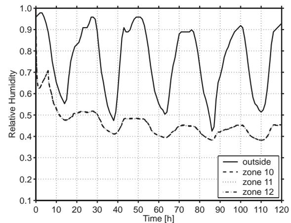
Figure 5 Relative humidity distributions vs. time for the hot and wet case
