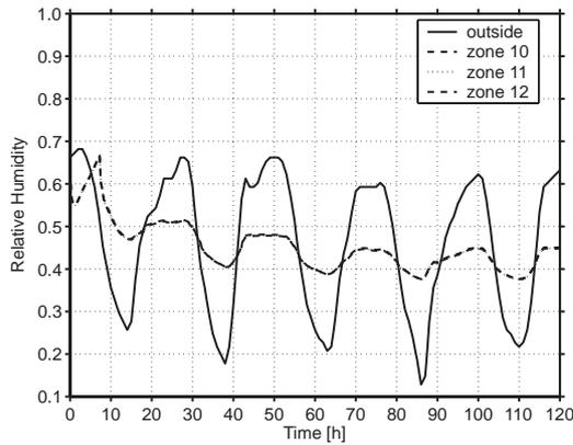
Figure 6 Relative humidity distributions vs. time for the hot and dry case
