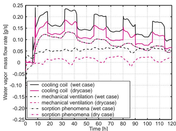
Figure 7 Net water vapor mass flow rate distributions vs. time due to cooling coil dehumidification, sorption phenomena and mechanical ventilation for humid and dry cases
