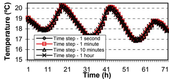
Fig. 9: Time step effects on room air temperature
