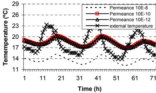
Fig. 11: paint vapor permeance effects on temperature
