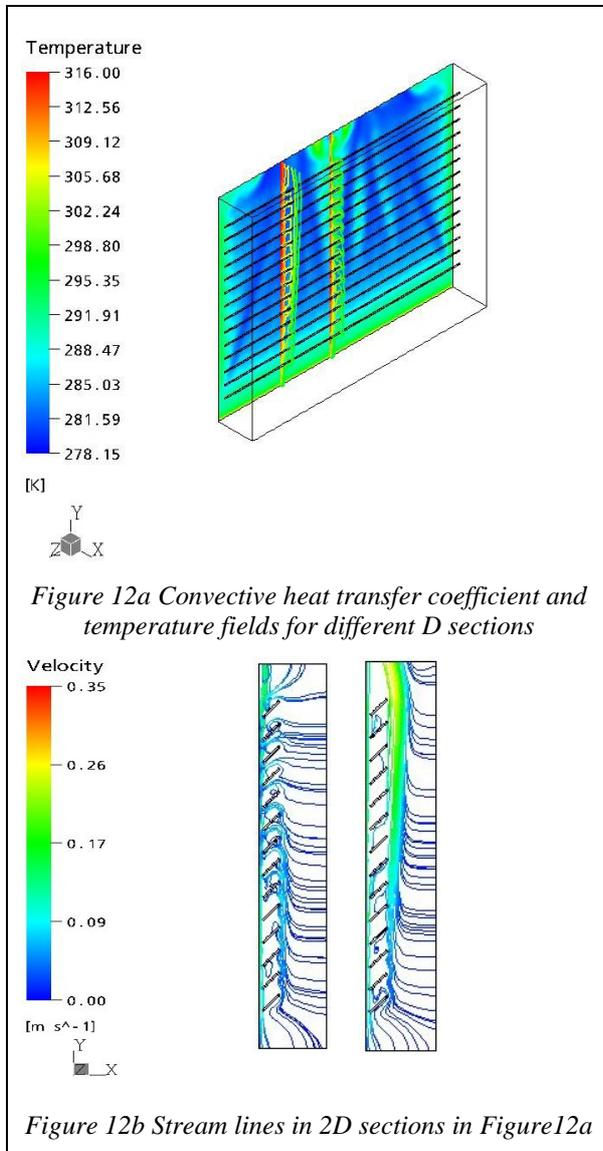
Figure 12 Dependence of 2D temperature and velocity fields on its position in 3D domain for summer conditions
