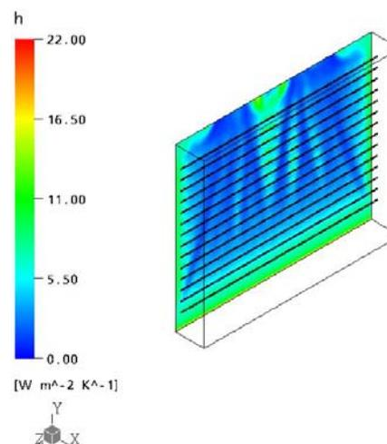
Figure 4b Wall heat transfer coefficients for partially closed ( $45^\circ$ ) blinds for summer conditions
