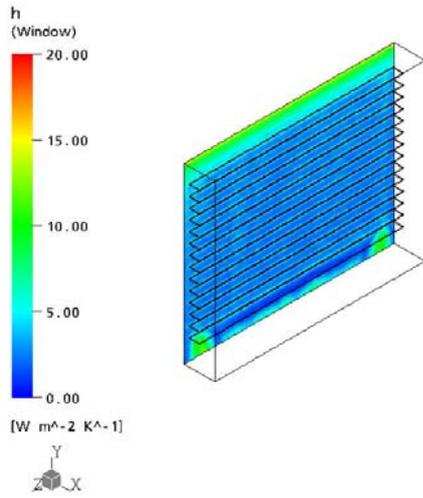
Figure 8a Wall heat transfer coefficients for open blinds for winter conditions
