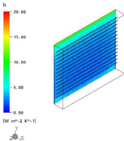
Figure 8b Wall heat transfer coefficients for partially closed (45°) blinds for winter conditions
