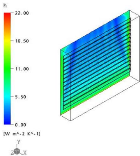
Figure 4c Wall heat transfer coefficients for closed blinds for summer conditions
