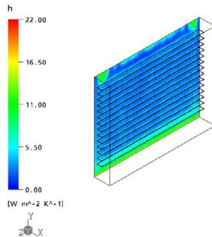
Figure 4a Wall heat transfer coefficients for open blinds for summer conditions
