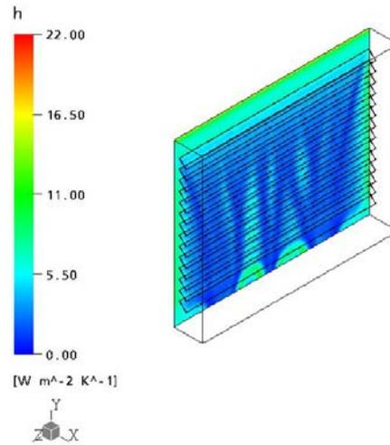
Figure 8d Wall heat transfer coefficients for partially closed (-45°) for winter conditions
