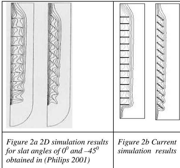
Figure 2 Temperature contours comparison for different slat angles
