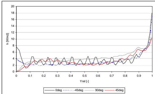
*Figure 11 Local convection heat transfer coefficients for winter conditions*
