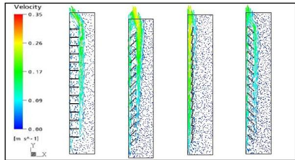
Figure 6 Velocity vectors for different slat angels for summer conditions
