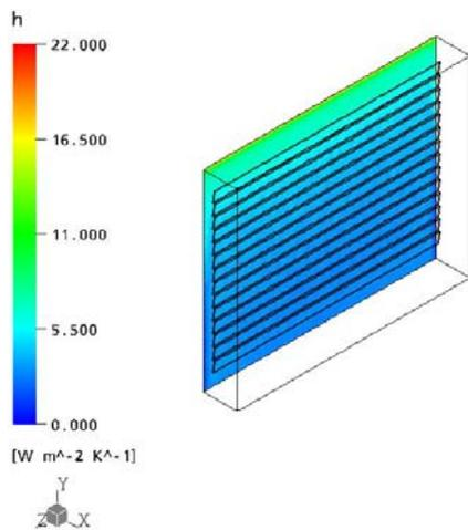
Figure 8c Wall heat transfer coefficients for closed blinds for winter conditions
