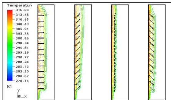
Figure 5 Temperature contours for different slat angles for summer conditions
