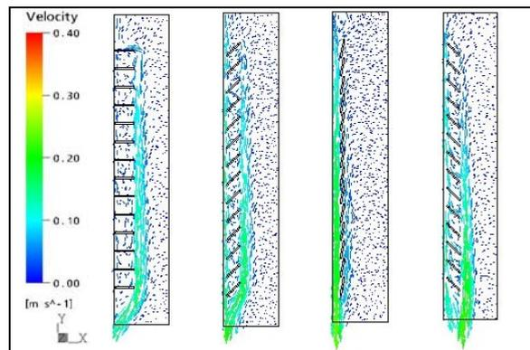
Figure 10 Velocity vectors for different slat angles for winter conditions
