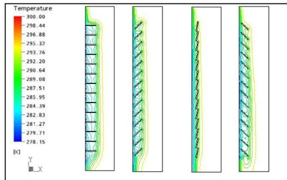
Figure 9 Temperature contours for different slat angles for winter conditions
