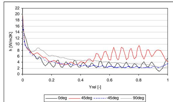
Figure 7 Local convection heat transfer coefficients for summer conditions
