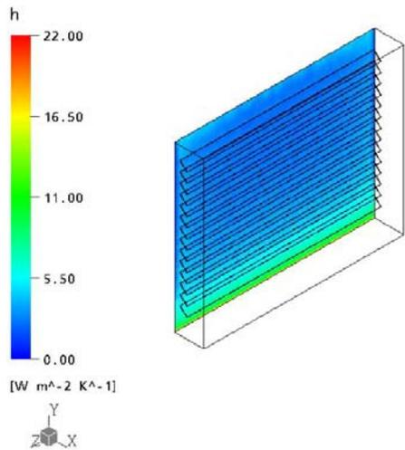
Figure 4d Wall heat transfer coefficients for partially closed (-45°) blinds for summer conditions
