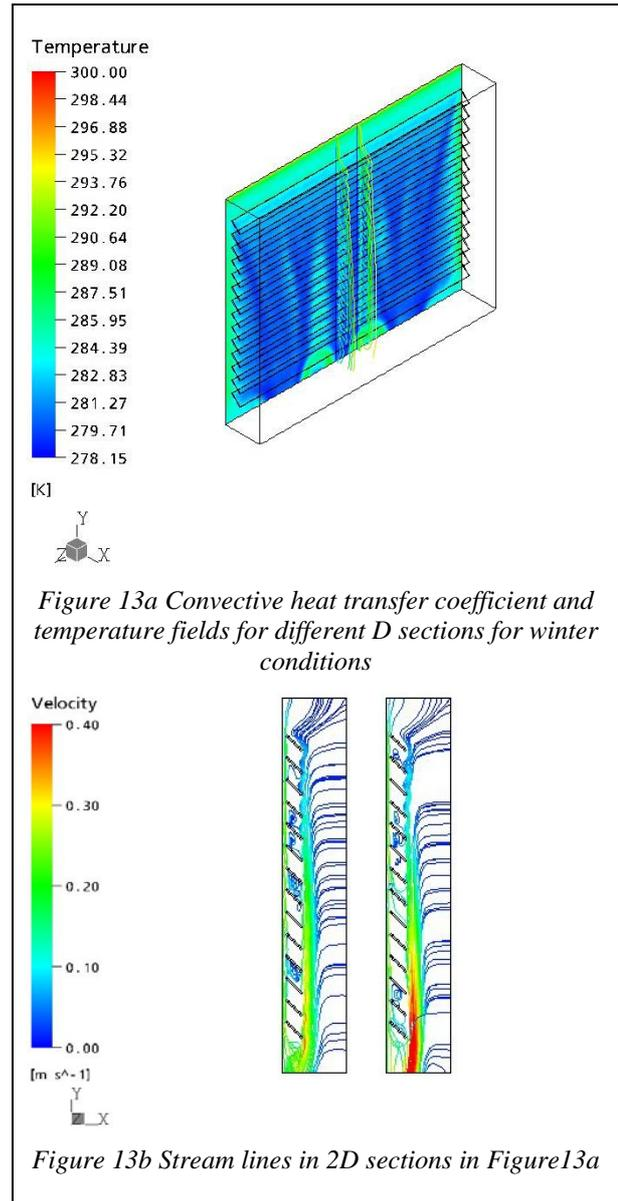
Figure 13 Dependence of 2D temperature and velocity fields on its position in 3D domain for winter conditions
