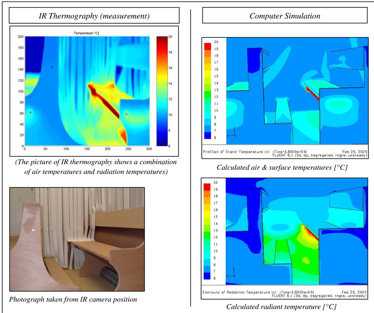
Figure 8. Qualitative comparison between measured temperatures (left) and calculated temperatures (right)
