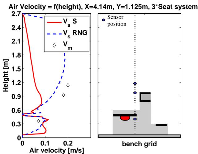
Figure 11. Comparison of air velocity over a vertical line at the back of the seat
