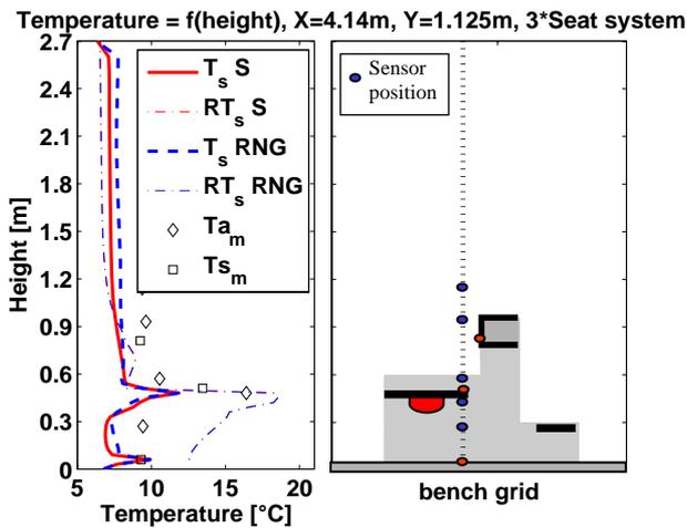
Figure 9. Comparison of temperatures over a vertical line at the back of the seat
