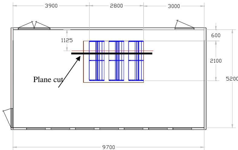
Figure 3. Overview dimensions (mm) of climate room, benches and plane cut.
