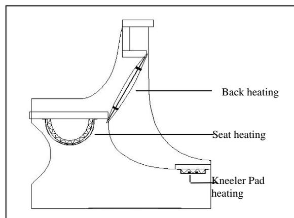
Figure 1. Position of the heating elements
