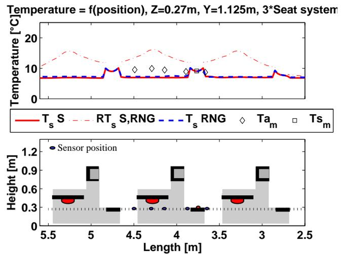
Figure 10. Comparison of temperatures over a horizontal line at kneeler pad height
