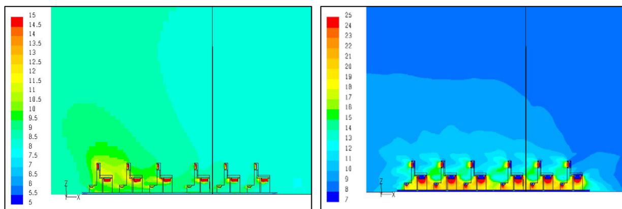
Figure 14. Air temperature [°C] (left) and radiant temperature [°C] (right) in / around the church benches.
