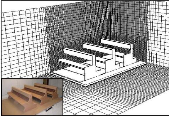
Figure 6. Climate room set-up: photograph and the CFD geometry with grid cell distribution.
