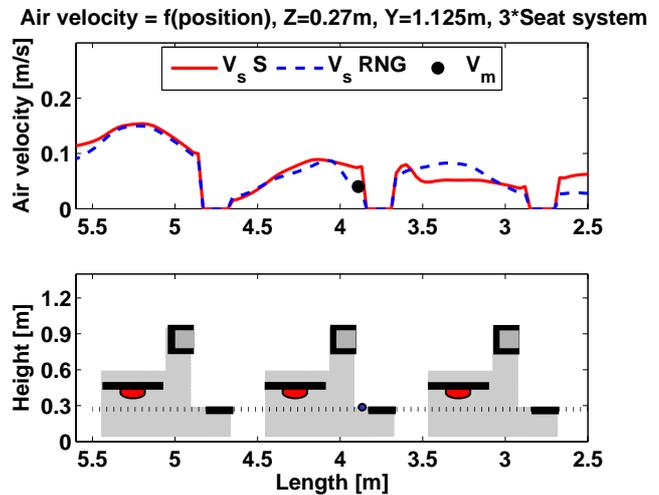
Figure 12. Comparison of air velocity over a horizontal line at kneeler pad height
