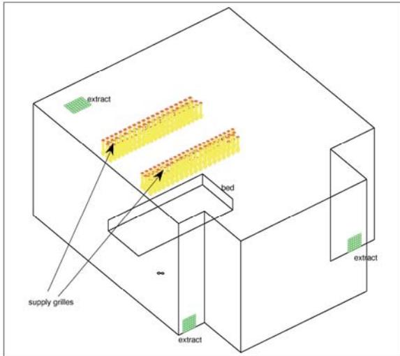
Figure 11 CFD geometry
