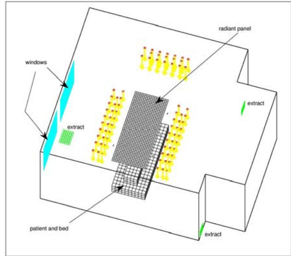
Figure 5 CFD geometry
