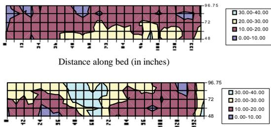
Figure 9 Airflow patterns for 600CFM at 70 F and no radiant panel
