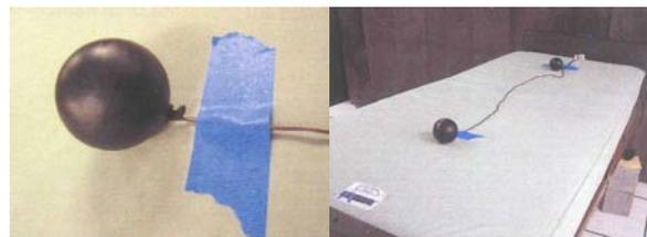
Figure 8 Radiant temperature sensor and arrangement on the bed
