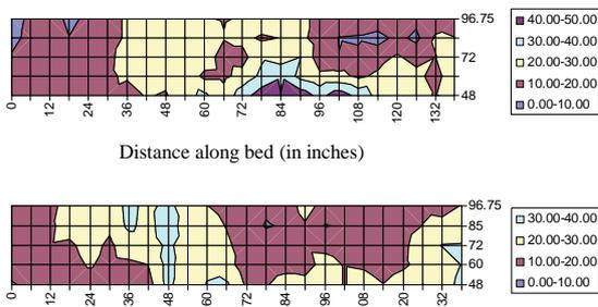
Figure 10 Airflow patterns for 600CFM at 70 F with radiant panel
