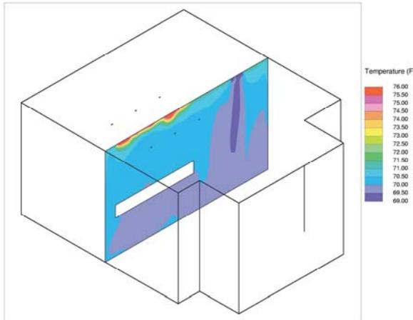
Figure 6 Velocity vectors and temperature contours
