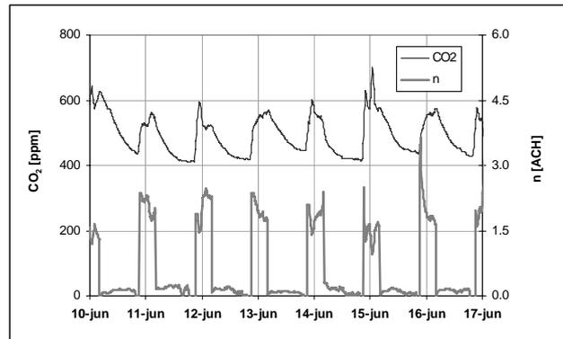
Figure 6 CO<sub>2</sub>-concentration measured (hourly average) and ventilation rate *n* calculated for the case of the room with the parallel window.
