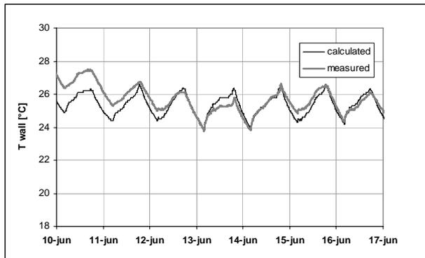
Figure 7 Calculated and measured indoor wall temperature for the case of the 'reference' room, where no night cooling is applied.
