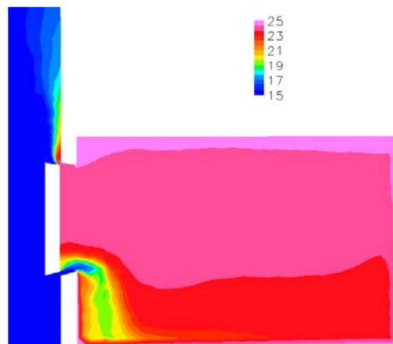
Figure 9 CFD simulation of the temperature distribution in the interior of the room with the **parallel window** in a plane perpendicular to the façade through the middle of the window. The rectangle on the left is part of the outside world at a temperature of 15°C.
