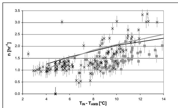
Figure 11 CFD calculations (solid lines) and measurements (symbols) of night cooling ventilation rate versus the difference between indoor and ambient temperature. Black line and black crosses: two panels, grey line and grey squares: parallel window. Error bars are due to the (estimated) effect of wind speed.
