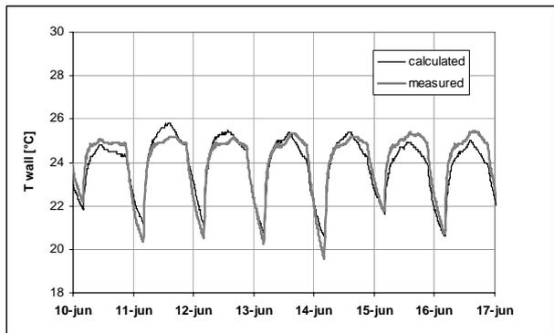
Figure 8 Calculated and measured indoor wall temperature for the case of the room with the parallel window, opened during the night.
