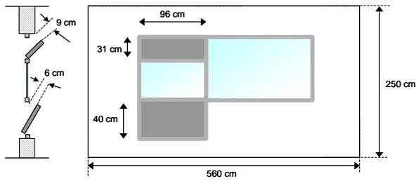
Figure 1 Cross section and front view of the façade with the two panels (shown in grey), opening to the inside.
