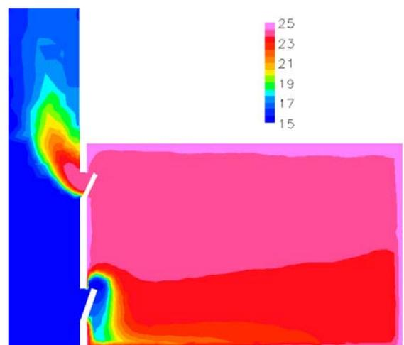
Figure 10 CFD simulation of the temperature distribution in the interior of the room with the **panels** in a plane perpendicular to the façade through the middle of the panels.
