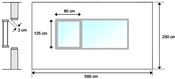
Figure 2 Cross section and front view of the façade with the parallel window, opening to the outside.
