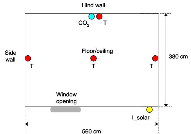
Figure 5 Floor plan of a room with the location of sensors. Sensors on the hind wall and side walls are placed at a height of 1.5m.
