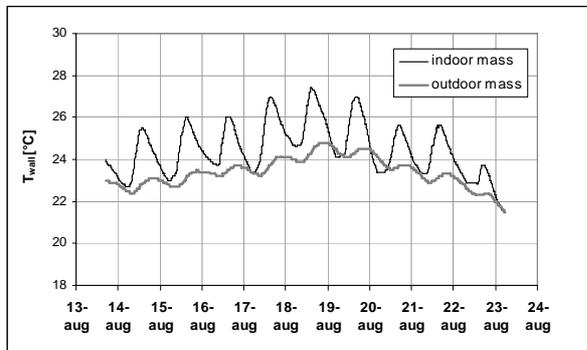
Figure 8 Variation of indoor and outdoor mass temperature, calculated for the case of room nr. 2.
