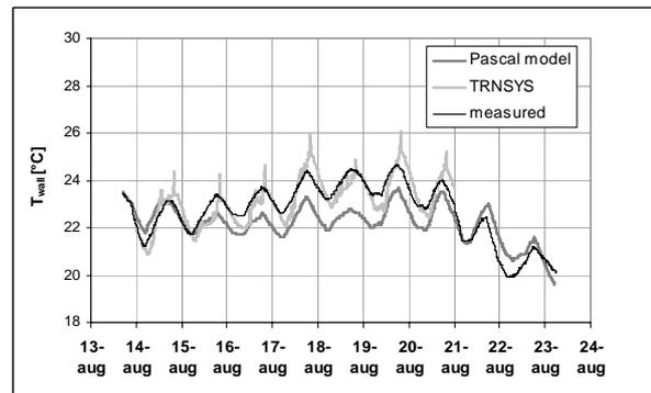
Figure 7 Calculated and measured indoor wall temperature for the case of room nr. 1, oriented towards the north, without night cooling.
