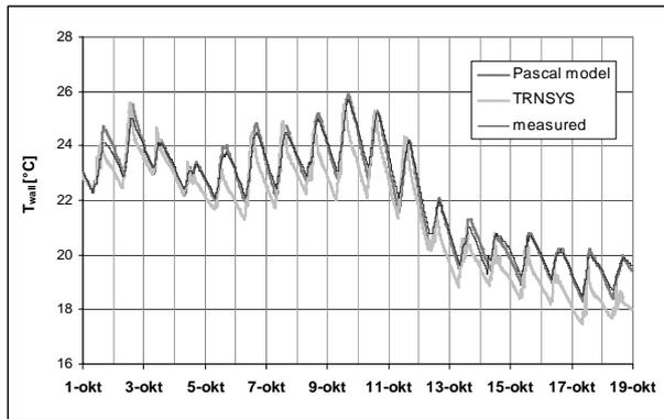
Figure 11 Calculated and measured indoor wall temperature for the Ecobuild A dwelling.
