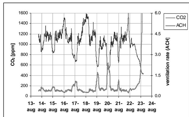
Figure 3  $\text{CO}_2$ -concentration measured and ventilation rate calculated (expressed in ACH). The drop in the  $\text{CO}_2$  concentration at the end is due to the draining of the  $\text{CO}_2$ -container.
