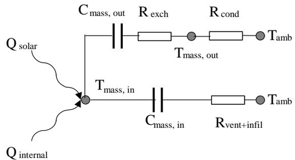
Figure 5 Three-temperature-node representation of the 'Pascal' building simulation model. The indoor mass temperature  $T_{\text{mass, in}}$  is connected through an RC-element to the ambient temperature  $T_{\text{amb}}$  and through another RC-element to the outdoor mass temperature  $T_{\text{mass, out}}$ . To the left are heat flows  $Q_{\text{solar}}$  and  $Q_{\text{internal}}$ .
