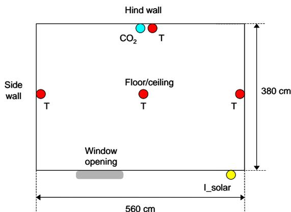
Figure 2 Floor plan of a room with the location of sensors. Sensors on the hind wall and side walls are placed at a height of 1.5m.
