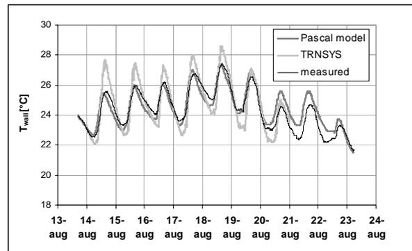
Figure 6 Calculated and measured indoor wall temperature for the case of room nr. 2, oriented towards the south. At night, the window was opened for night cooling.
