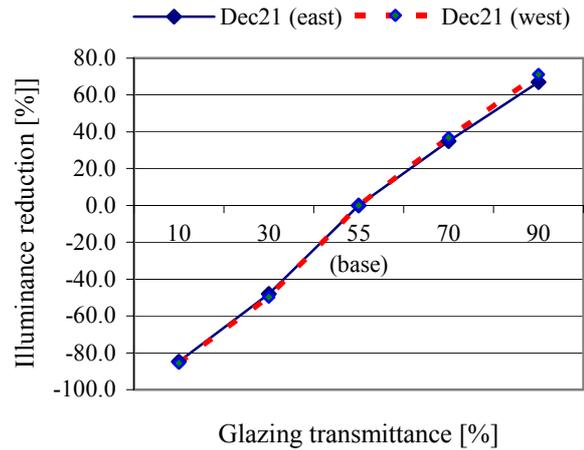
Figure 11. The impact of glazing transmittance on the reference point illuminance
