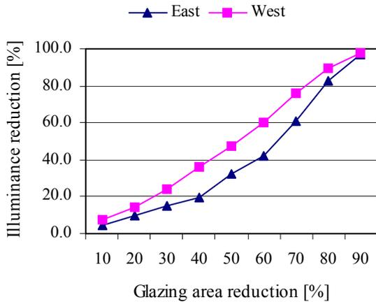
Figure 8. The impact of glazing area reduction on reference point illuminance in Dec.
