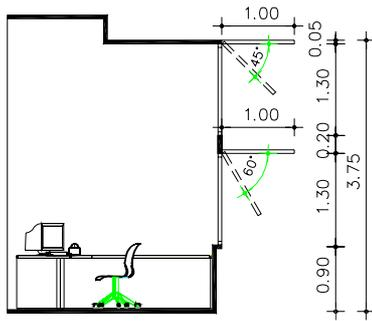
Figure 13. Section of the window wall for the final alternative
