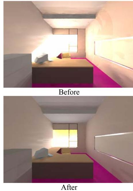
Figure 7. The impact of using movable overhang on glare control
