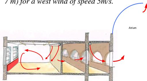
Figure 7 Air flows when the wind pressure on the outer facade is too high
