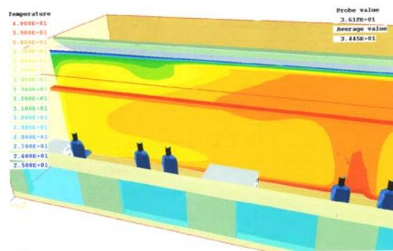
Figure 12 Temperature distribution in the roof-level rooms under summer conditions
