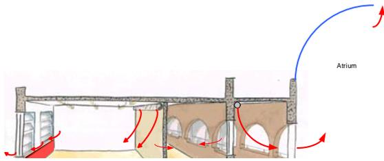
Figure 2 Working of the overpressure ventilation system
