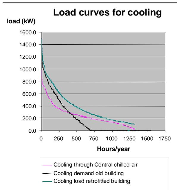
Figure 5 Load curves for the cooling demand
