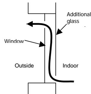
Figure 8 Exhaust air system
