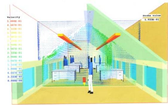
Figure 11 Air flows and velocities in the roof-level rooms under summer conditions
