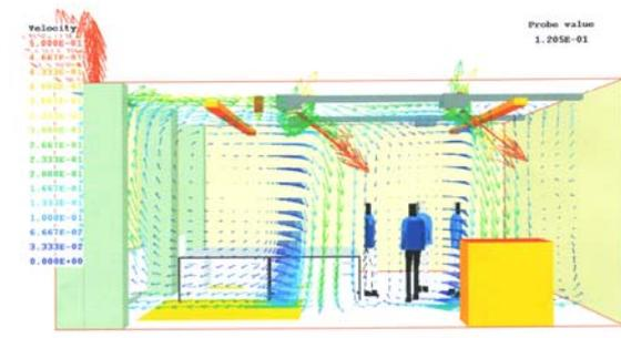
Figure 13 Air flows and velocities in the first-floor rooms
