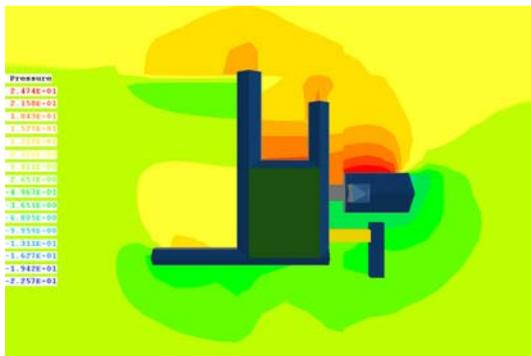
Figure 6: Wind pressure distribution ( height 7 m) for a west wind of speed 5m/s.
