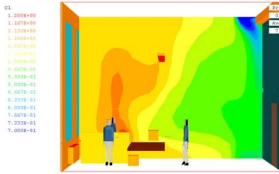
Figure 10 Dispersion of breathing air when the exhaust vents in the façade are closed
