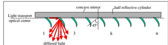
Figure 5 Diagram of optical model of the light pipe.
