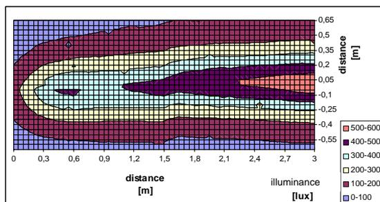
Figure 8 Isolux Curves – lux-meter photometrical characterization (half light pipe).
