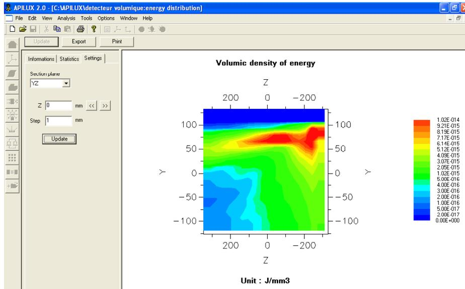
Figure 14 Distribution of light on a lateral wall.
