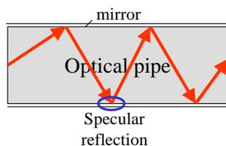
Figure 1 The first mirror light pipe.
