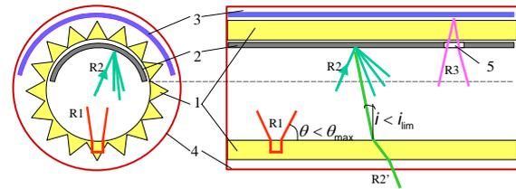
Figure 4 Inner section of the light pipe and the different light ways .
