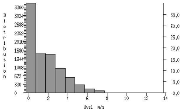
Figure 4: Frequency histogram of annual wind speed.
