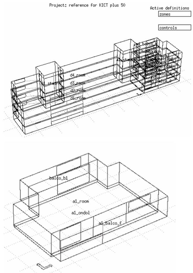
Figure 8: ESP-r model of the PLUS 40 building.
