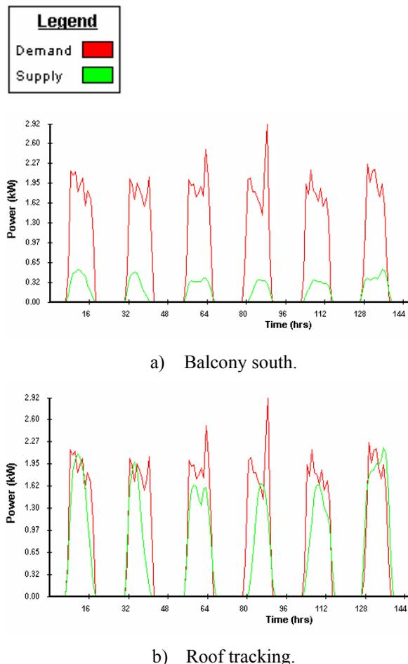
Figure 10: Graphic results of matching analysis for PV options (8/4-13/4).
