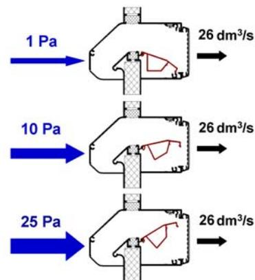
Figure 3 Self-regulating air inlets
