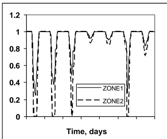
Figure 1. Lighting power multipliers for ZONE1 with window and ZONE2 with upward-redirecting CFS.
