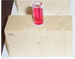
Figure 10. Wood sample subjected to point wetting from the top.
