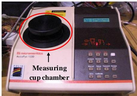
Figure 4. Pycnometer AccuPyc 1330TC by Micromeritics©
