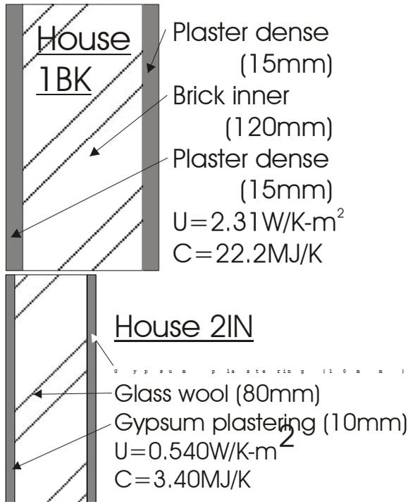
Fig.3 the composition of the partition assembly for different houses 1BK and 2IN
